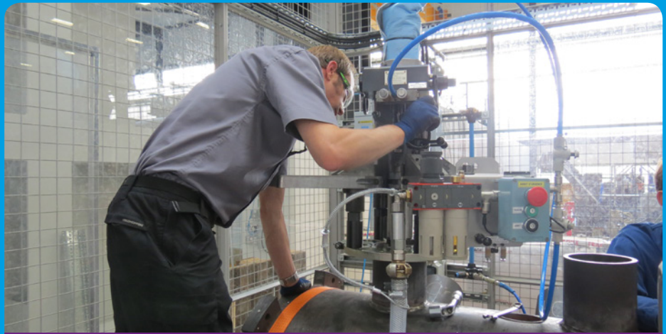
Flexible friend: setting up a portable machine tool in the Nuclear AMRC test cell.
