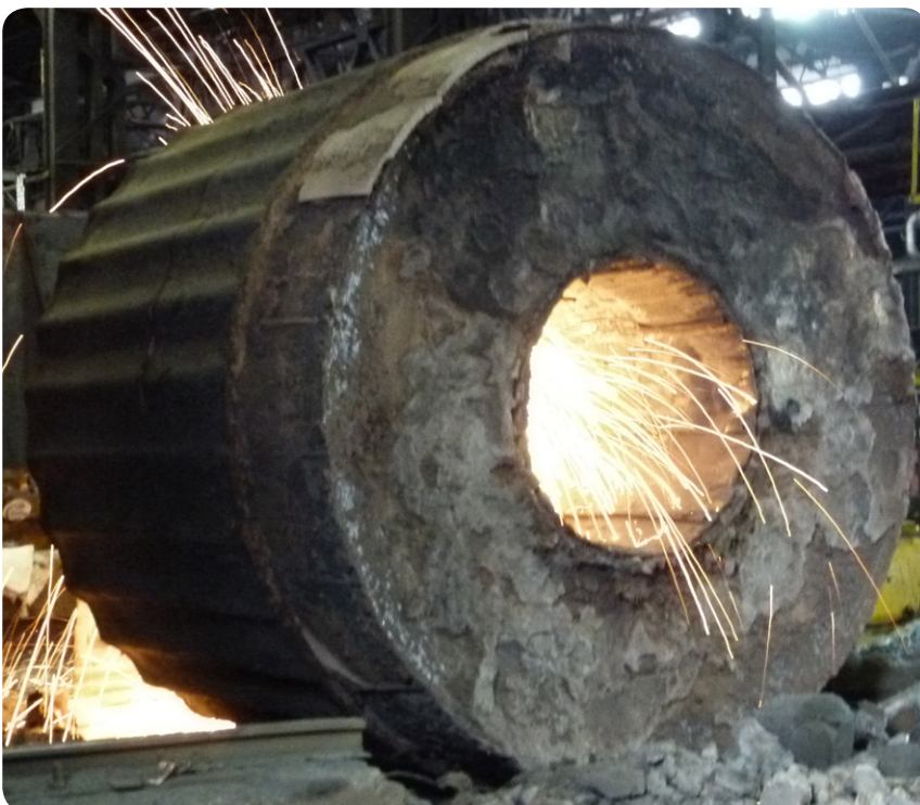
Hollow ingots allow more efficient forging of large nuclear components.
