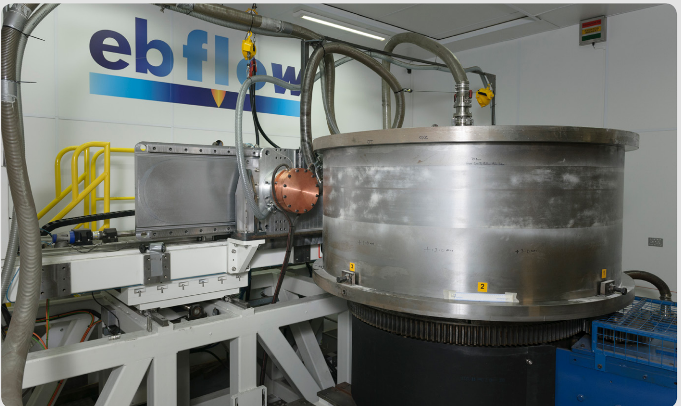
Welding trials on CVE's EBFlow machine.
