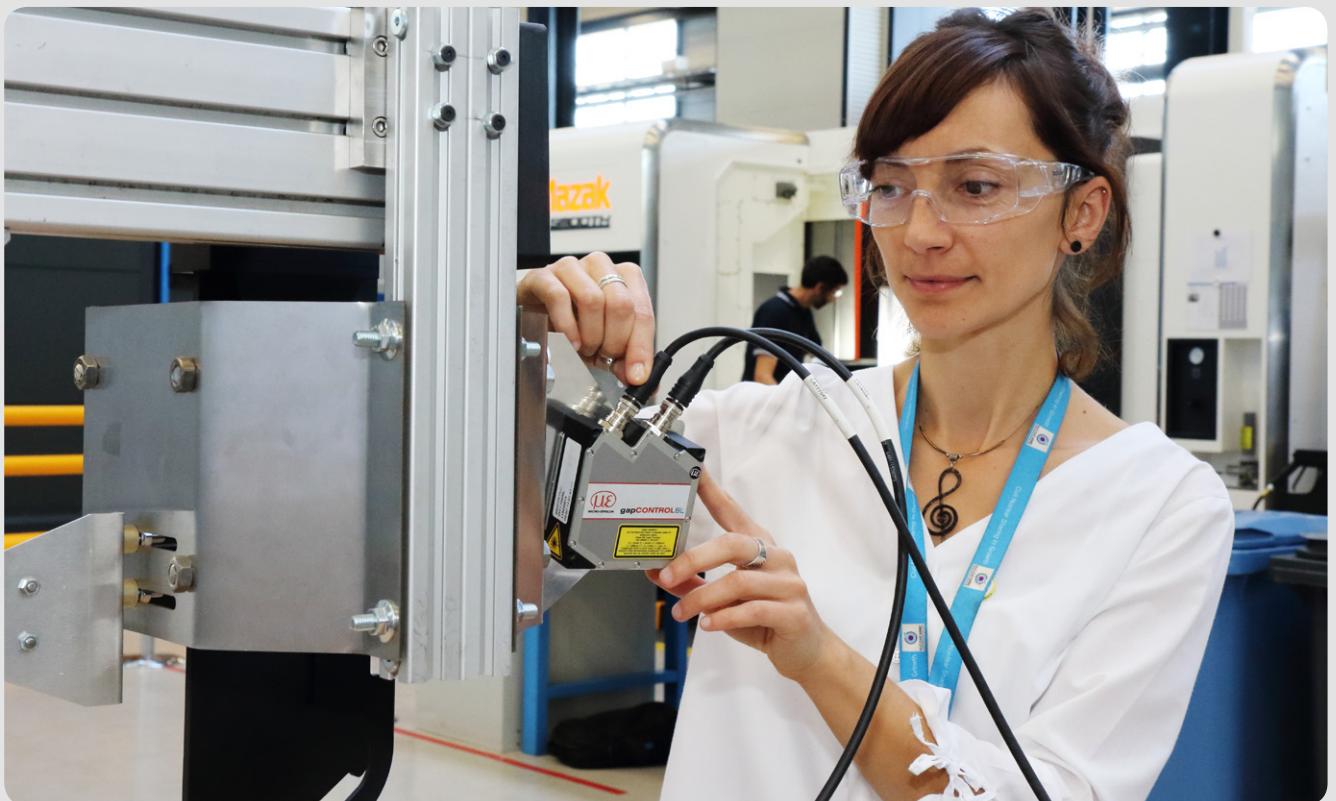
A 3D-printed replica of the Polysoude welding head used to optimise sensor positioning.
