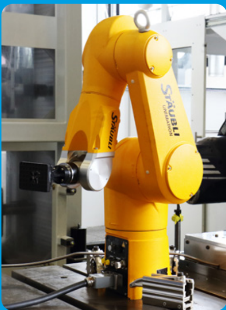
Helping hand: the Nuclear AMRC team integrated a small robot arm with the Soraluece machining platform to support a workpiece.
