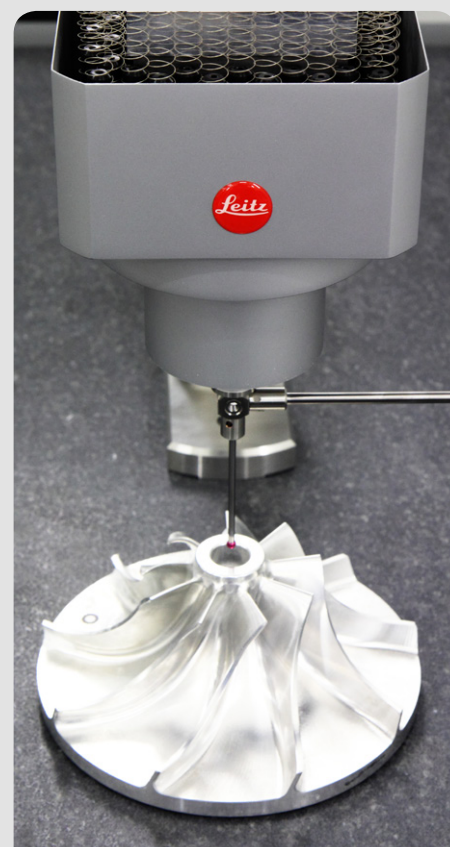
Ultra-precision: the new Leitz CMM is capable of sub-micron resolution of large parts.
