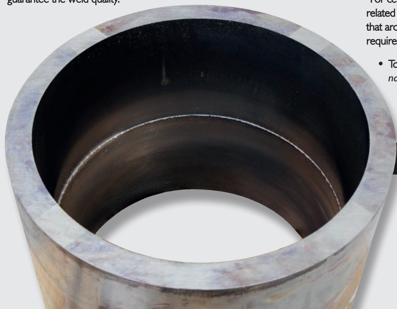
Four-minute milestone: demonstration weld on 600mm pipes.
