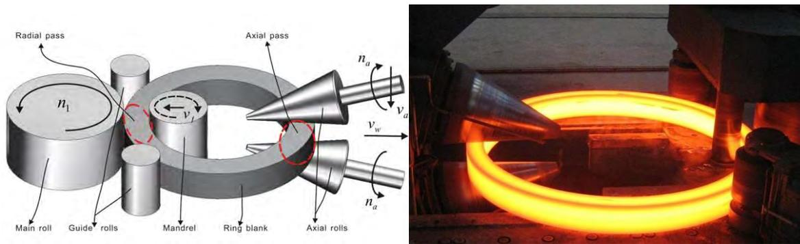
Figure 65: The process of ring rolling
