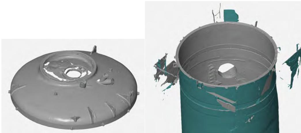
Figure 21: Laser scan of a vacuum chamber and closure head used for vacuum stream degassing at SFIL
