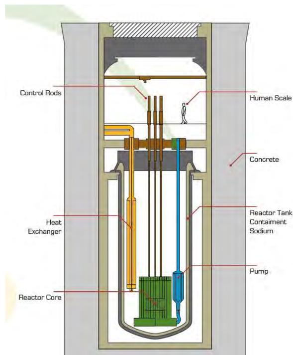
Figure 3: The ARC 100 Reactor
