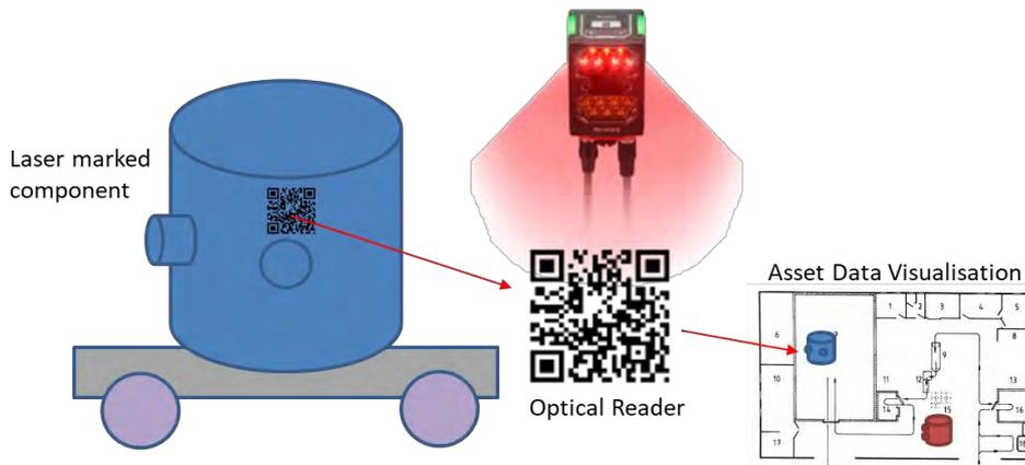
**Figure 3: System Concept: Asset Tracking**
