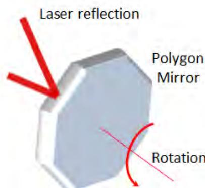
**Figure 2-8 - Single laser beam passing through a rotating polygon mirror.**
