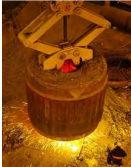
Figure 50: Ingot striping of 160-metric ton casting prototype was the result of more than a year of investment and development at Sheffield Forgemasters.
