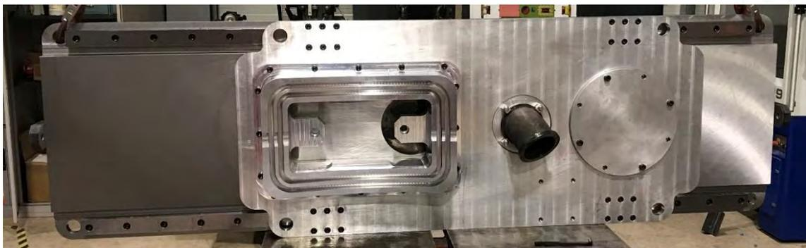
**Figure 3 Front view of the static seal plate (front), sliding seal plate (back). Shown without sliding seal, fronting bar and beam dump in place.**
