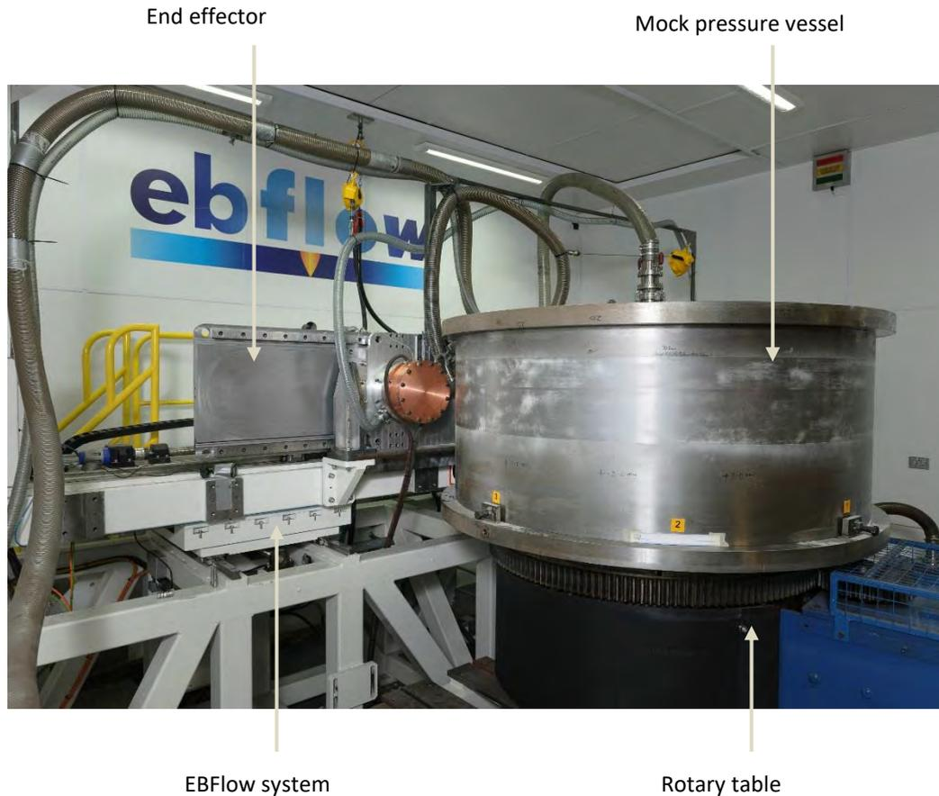
**Figure 3 InFORM equipment integrated with CVE's EBFlow system.**
