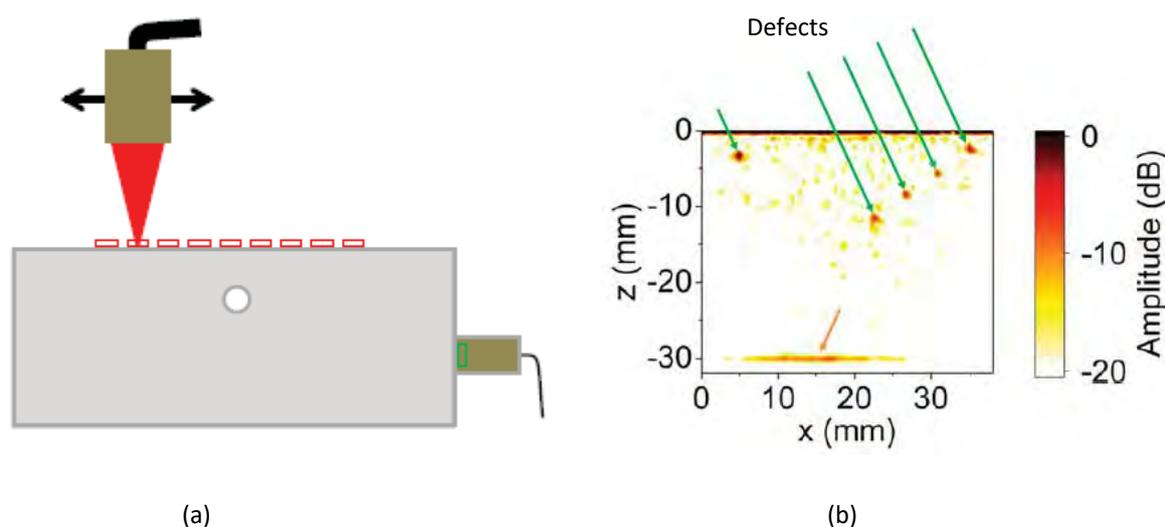
**Figure 7-3: Hybrid laser ultrasonic developed by Bristol University (a) schematic diagram (b) improved signal processing to enhance sensitivity**
