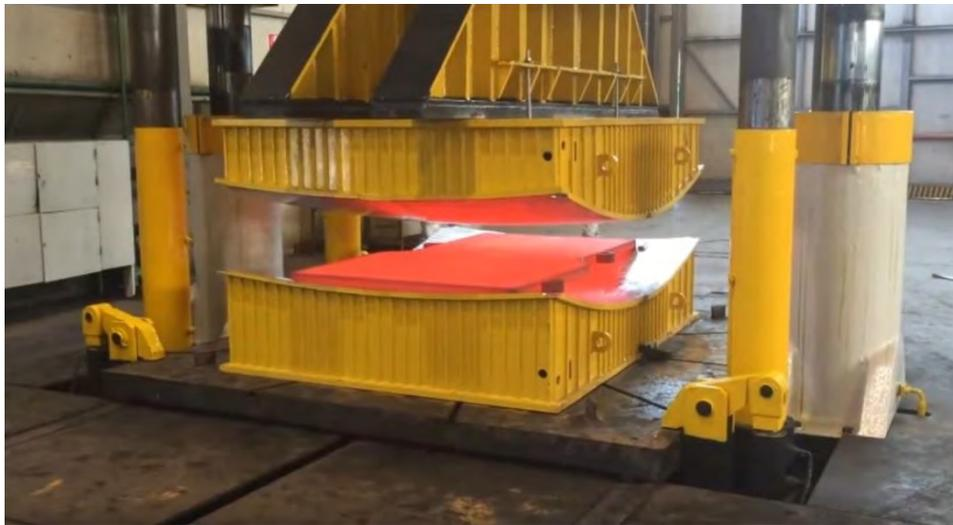
Figure 64: Hot forming of the ITER fusion reactor vacuum vessel using lightweight sandwich-type tools made of 316L (N)
