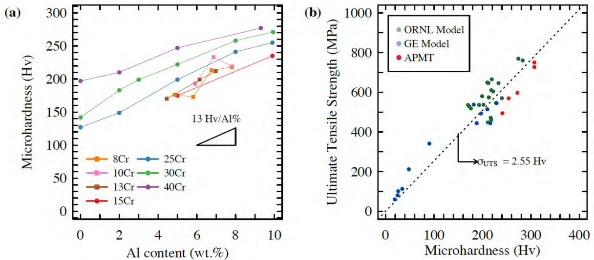
Figure 31: Room temperature hardness values for model FeCrAl alloys. a) Cr and Al effect on microhardness and b) simple property-property correlation between ultimate tensile strength and microhardness for unirradiated FeCrAl alloys [42]
