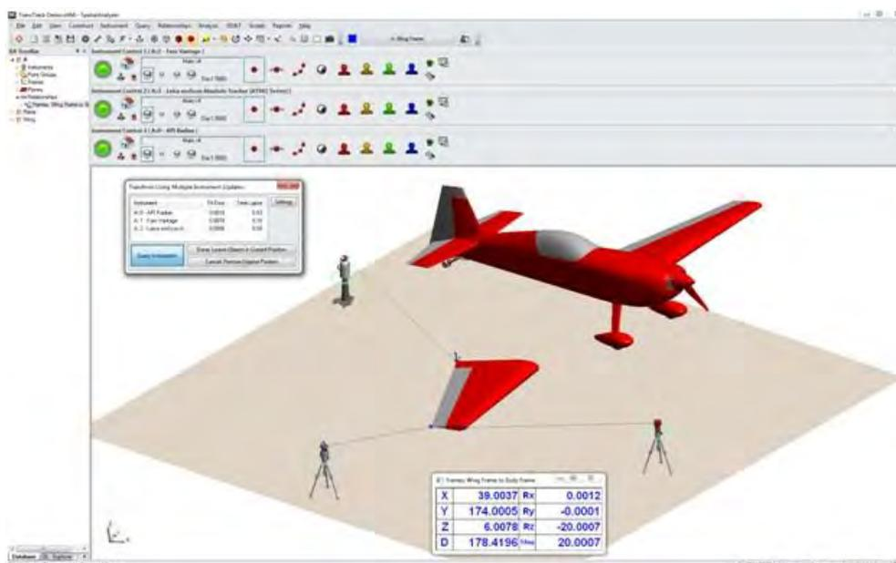
**Figure 5-2: Spatial Analyser software showing six degrees of freedom tracking of a component using three laser trackers**
