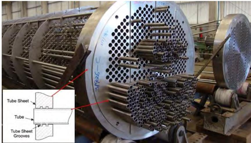
Figure 19: Tubesheets-tubes assembly
