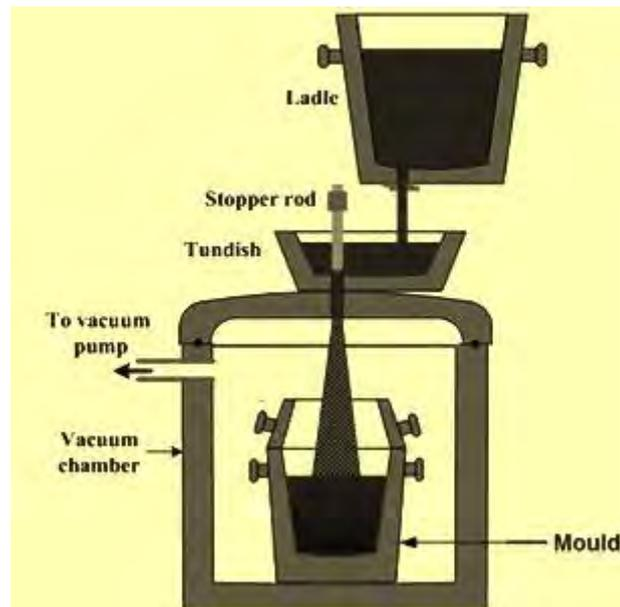
Figure 22: Schematics of ladle to mould degassing. The addition of the tundish is usually not necessary
