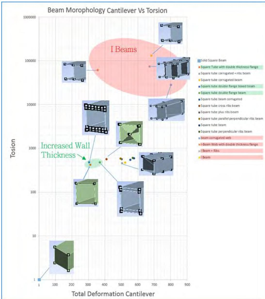
Figure 6 – Comparison Study of Beam Structural Morphologies
