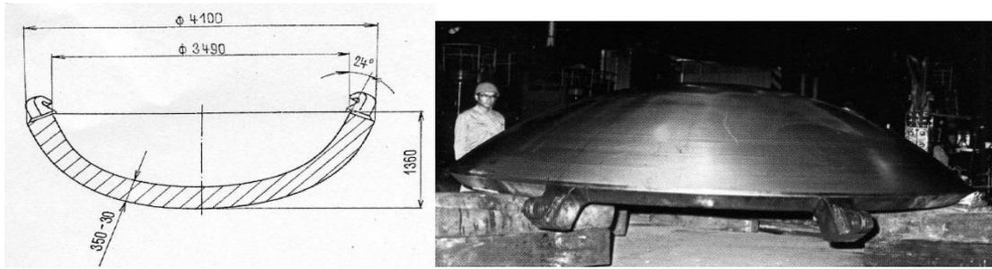
Figure 17: Drawing and pressed piece for the bottom of the reactor vessel [11]
