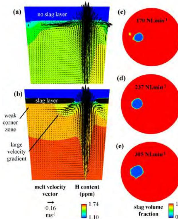
Figure 26: Molten steel flow field and hydrogen distribution across side profile plane after 20 minutes of vacuum degassing for (a) slagless and (b) slag-containing melt. Volume fraction of slag eye viewed from top profile after 20s of argon stirring for argon flowrates of (a) 170, (b) 237 and (c) 305NLmin<sup>-1</sup>
