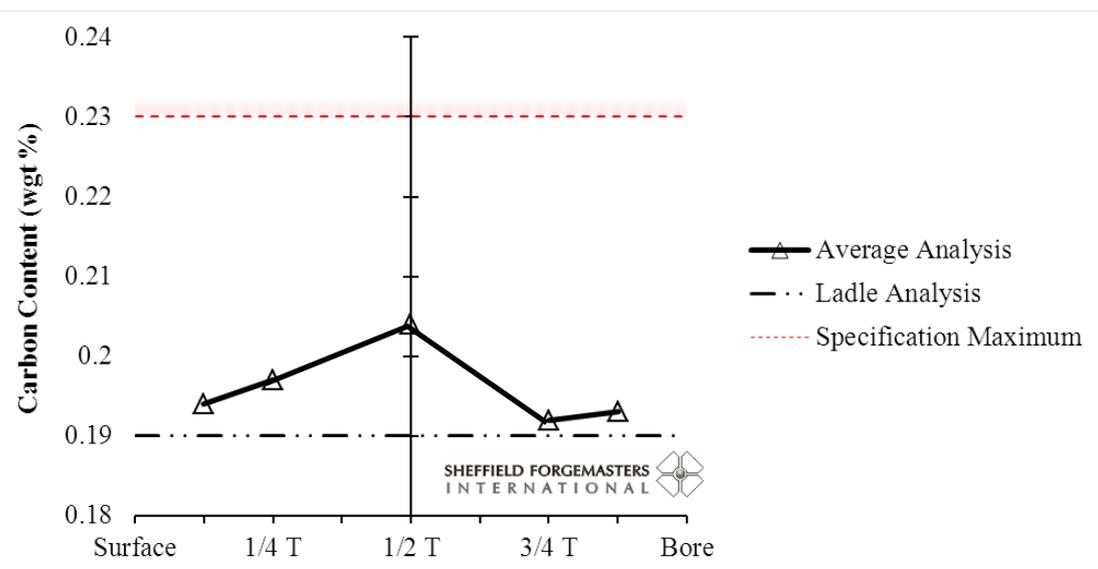
Figure 52: Plot of transverse carbon segregation pattern [78]
