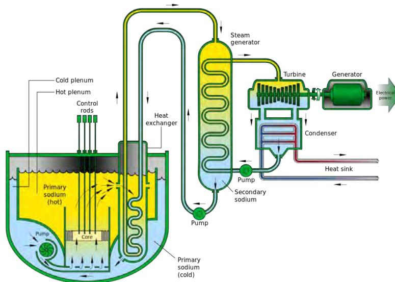
Figure 2: Schematic of the sodium-cooled fast reactor [5]
