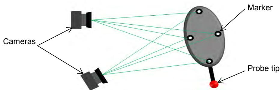
**Figure 2-3 - Illustration of an optical tracking system**
