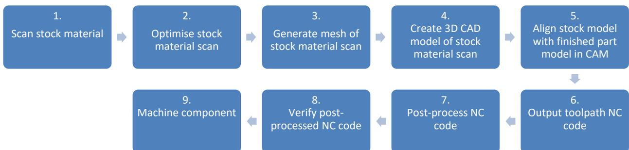
**Figure 3-11: Advanced reverse engineering workflow stages**
