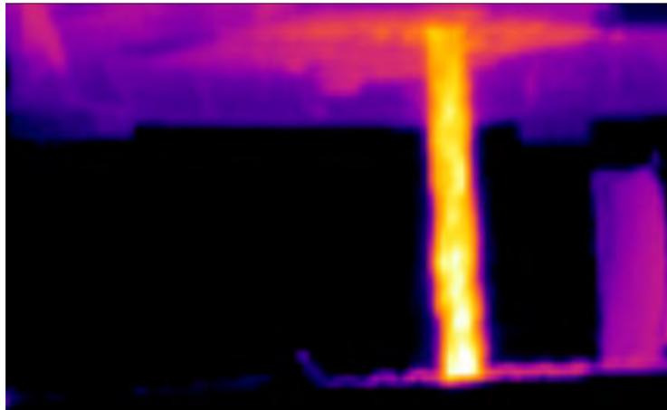
Figure 24: IR camera image used for temperature measurement during ladle pouring
