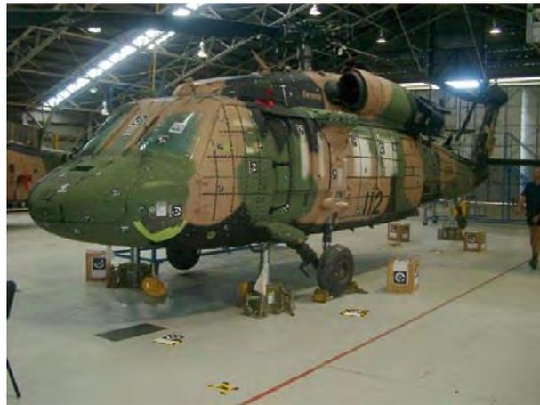
**Figure 1-1: Fuselage prepared for scanning (5)**
