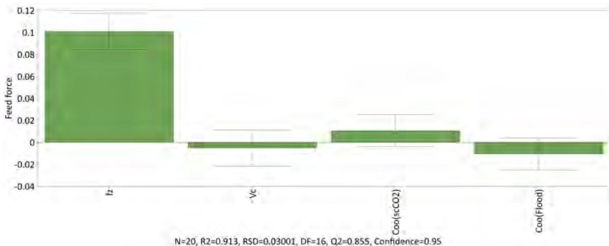
**Figure 3-14: The scaled and centred coefficients of the fitted model for the feed force in milling SA508**
