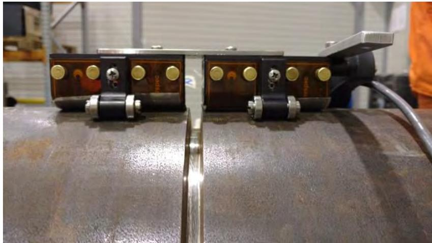
Figure 7-5: Innerspec temate<sup>®</sup> IWW system for in-process inspection
