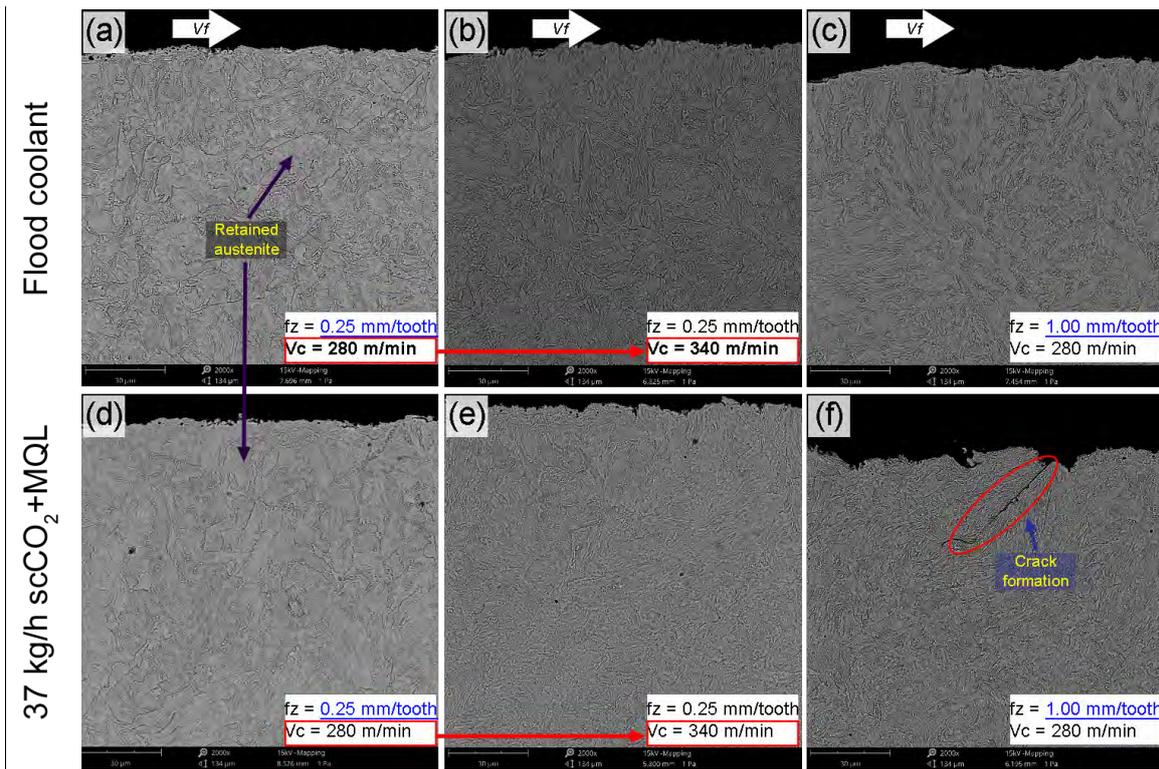
Figure 3-19: SEM micrographs (x2000) of the microstructures along the feed direction (longitudinal)
