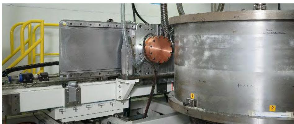
**Figure 6 End effector operating in QA position during dynamic vacuum tests.**
