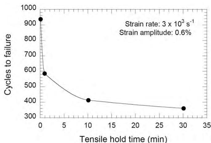
Figure 44: Effect of hold time on the fatigue life modified 9Cr-1Mo steel in air at 600°C [72]
