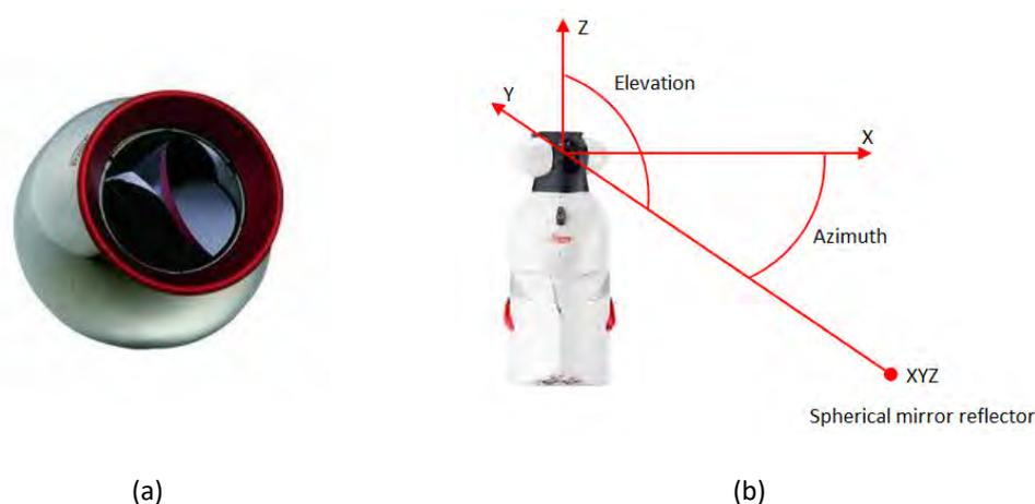
**Figure 2-1 – Spherically mounted reflector (a), Laser tracker co-ordinate system (b) (5)**
