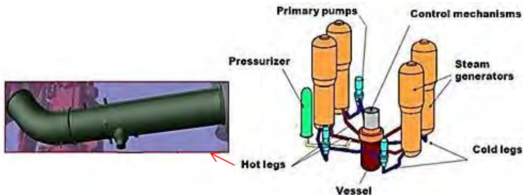
Figure 20: The hot leg (right) and the PWR Primary Circuit (left)
