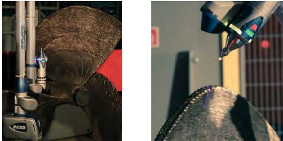
**Figure 1-4: 3D scan technology used in WAAM of ship propeller blades (6)**
