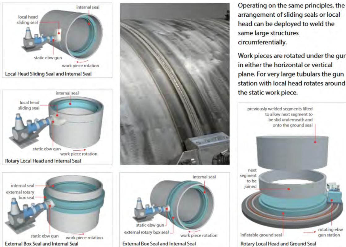
Figure 3-4: EBFLOW configurations for circumferential welding of tubular sections <sup>21</sup>
