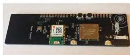
**Figure 6: Tiera Corp Long Cricket LoRaWAN processor module**
