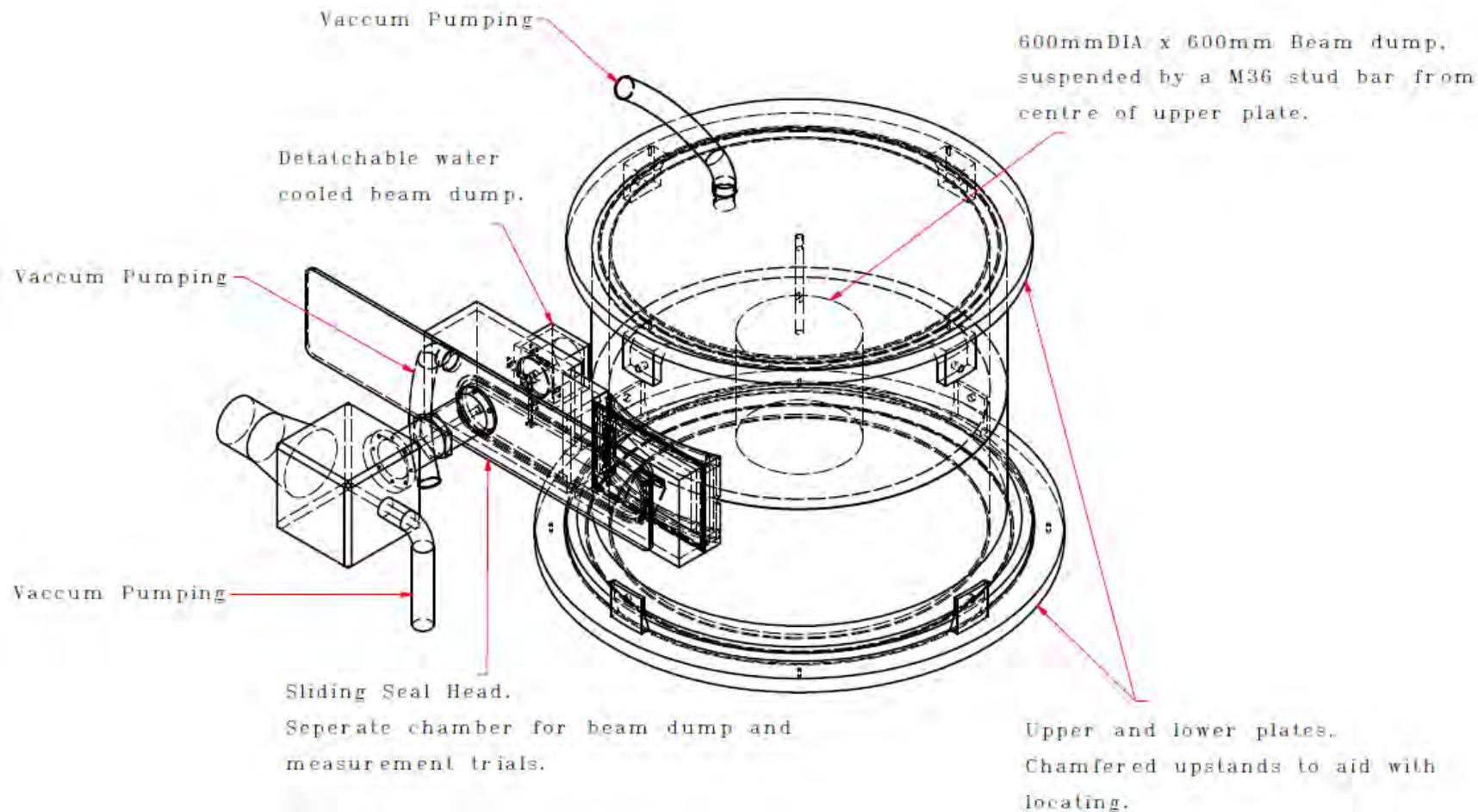
**Figure 3 Annotated wire-frame diagram of the system indicating key elements.**
