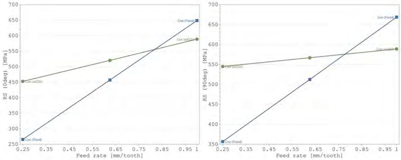
Figure 3-16: Interaction plot for the residual stress in the longitudinal (left) and transverse (right) directions
