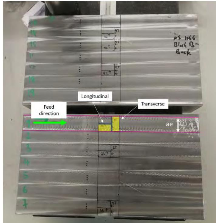
**Figure 3-18: SA508 workpiece before cutting into samples for microstructural analysis (*ae* is the radial depth of cut, *ae* = 20.4 mm)**
