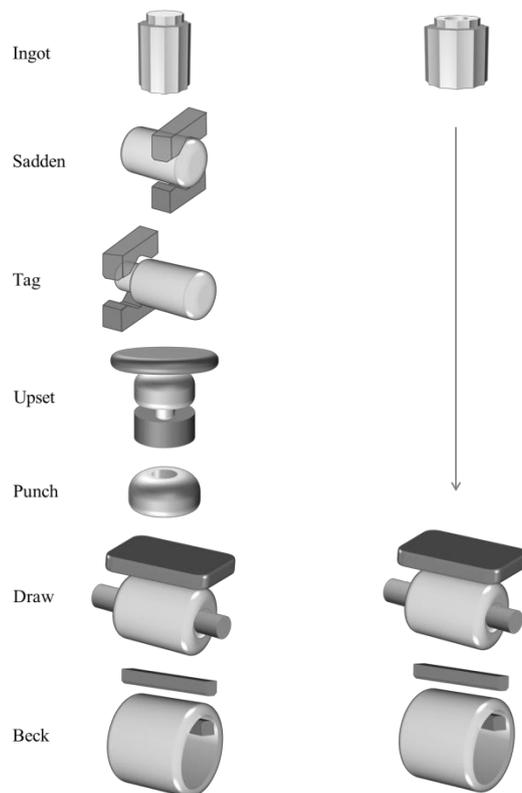
Figure 49: The conventional cylindrical forging route compared to that of the hollow ingot
