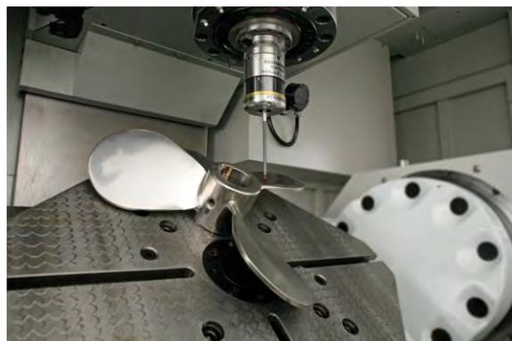
**Figure 4-1: RMP600 Strain gauge probe (26)**
