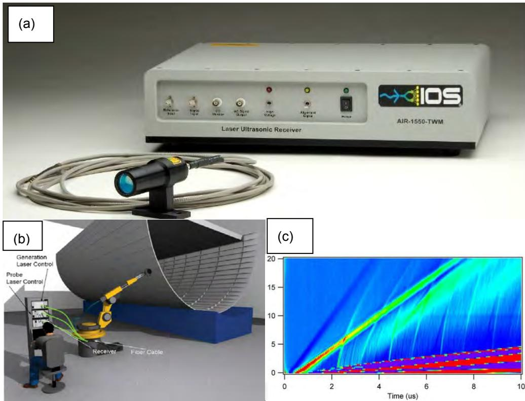
**Figure 7-4: Optech laser ultrasonic system (a) AIR-1550-TWM system (b) schematic drawing of agile measurement system (c) separation B-scan on a 6 mm steel sample**
