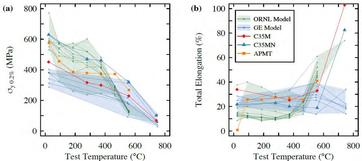
Figure 30: Yield strength and total elongation properties for select FeCrAl alloys as a function of temperature
