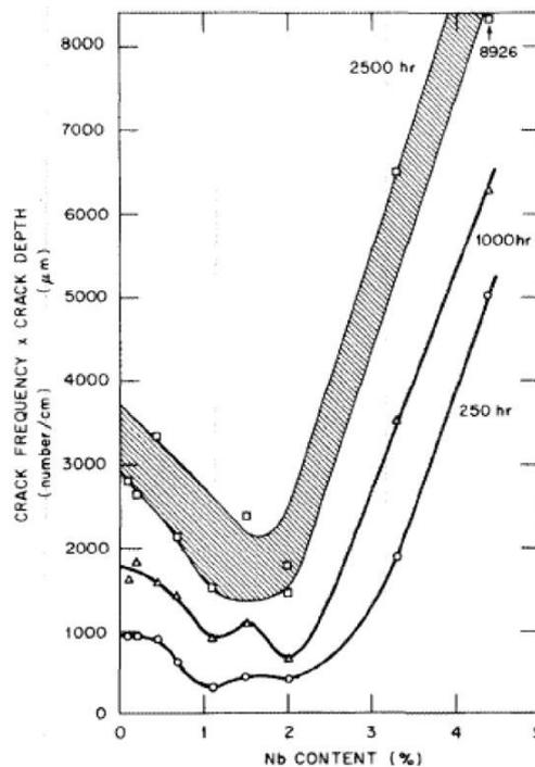
Figure 37: The influence of Nb content on cracking frequency in modified Hastelloy N
