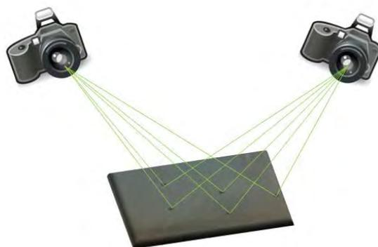
**Figure 2-11 – Illustration of how multiple locations of camera image can be combined and point positions calculated.**
