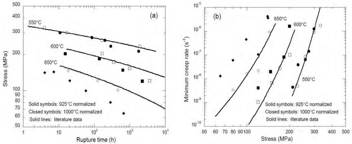
Figure 41: Creep rupture behaviour of modified 9Cr-1Mo steel normalized at 925 and 1050<sup>o</sup> [69].
