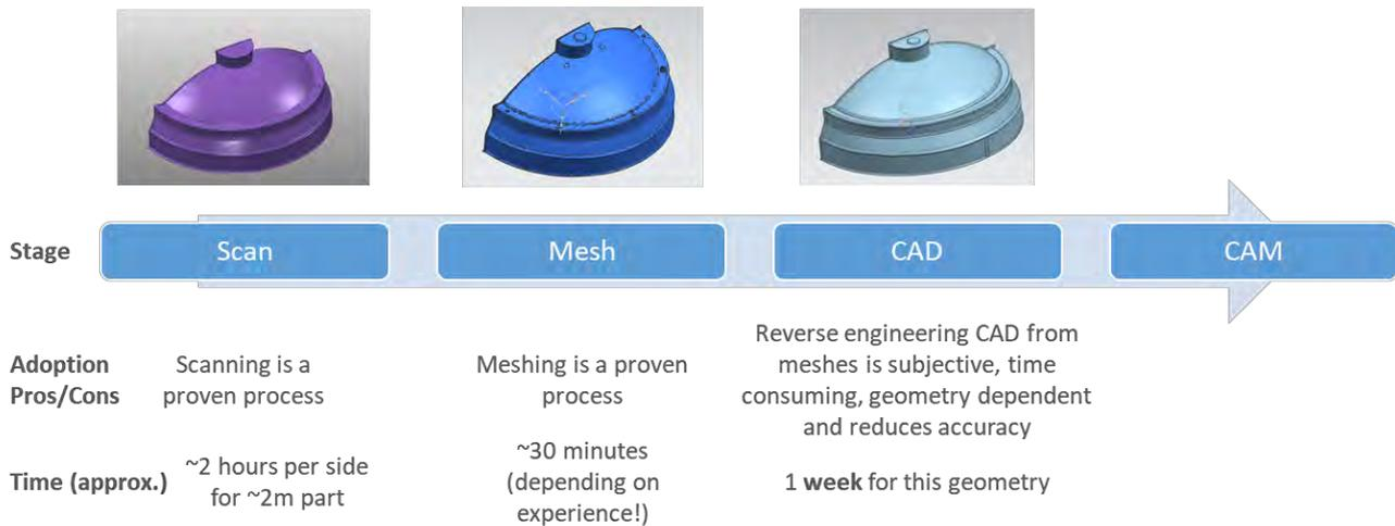
**Figure 3-10: Typical procedure in advanced reverse engineering**
