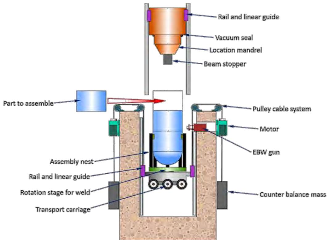
Figure 2 – The InFORM Vertical Silo-Build Concept - Diagram
