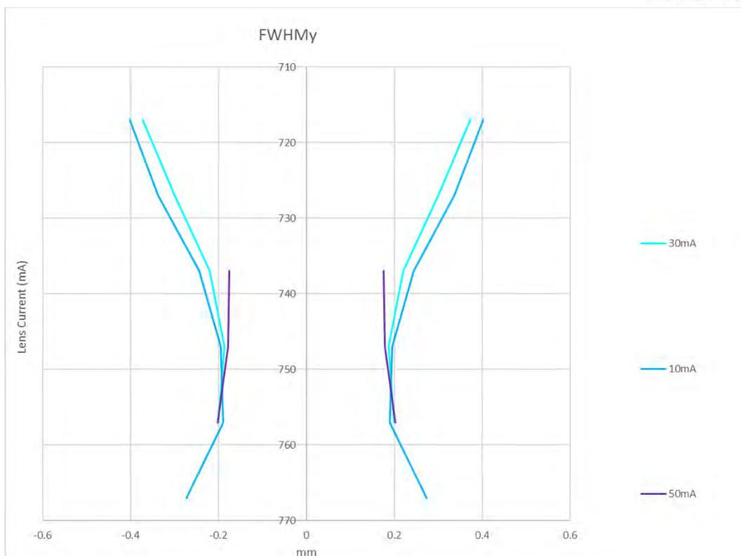
**Figure 21 Lens current vs FWHM Y.**
