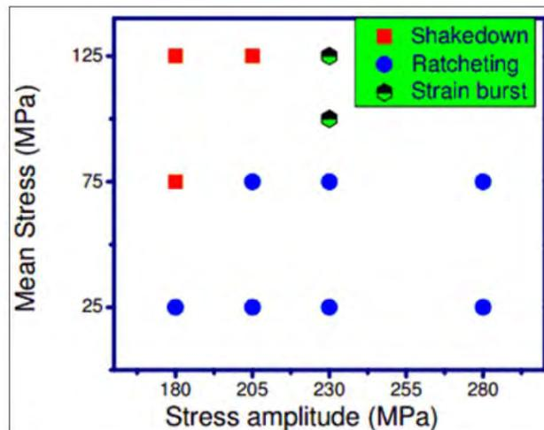
Figure 34: Influence of dynamic strain aging on ratcheting behaviour of 316L(N) austenitic stainless steel [50]. Elastic “shakedown” stands for elastic deformation
