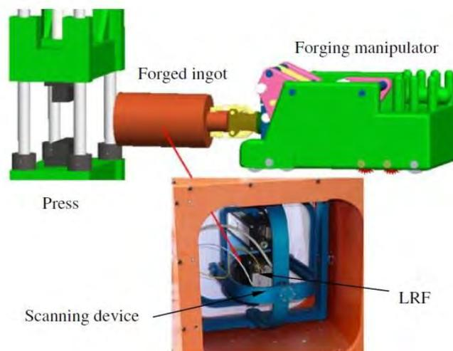
Figure 55: Scheme diagram of the measurement system
