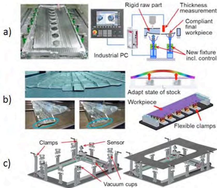
**Figure 3-2: (a) clamping force compensation; (b) residual stresses compensation; (c) toolpath correction<sup>19</sup>**
