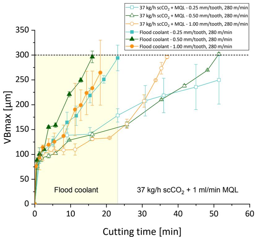
Figure 3-6: Maximum flank wear (VBmax) as a function of cutting time at various feeds and cutting speed of 280 m/min
