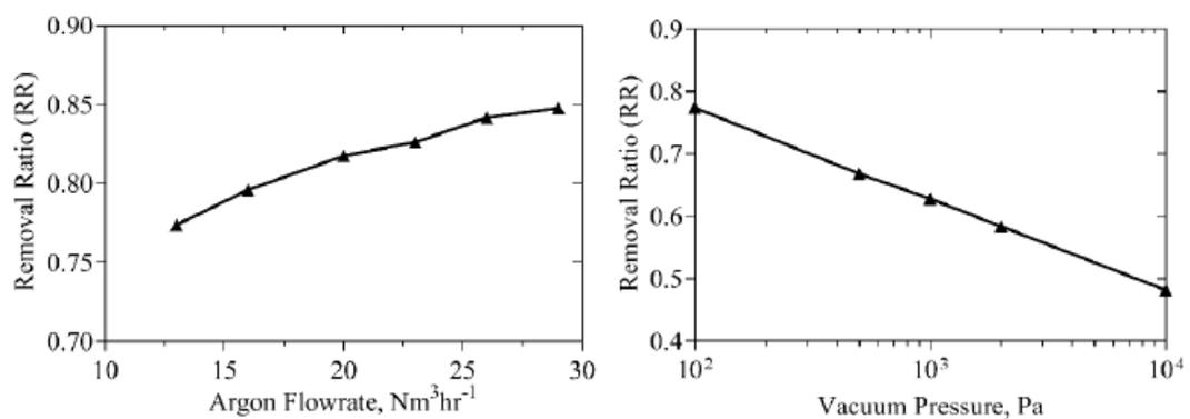
Figure 25: Variation of hydrogen removal ratio (RR) with argon flowrate and vacuum pressure
