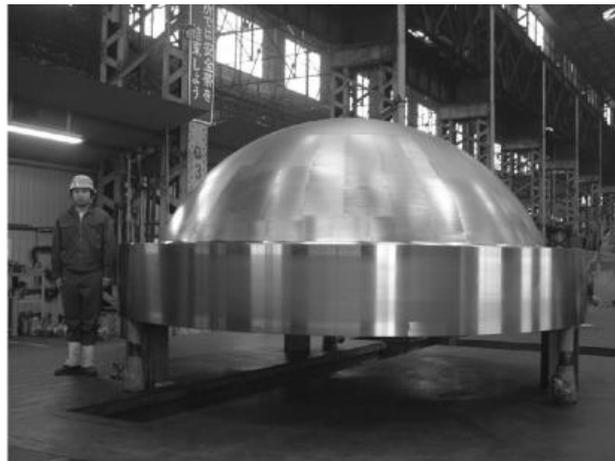
Figure 18: The closure head with integrated flange of a European Pressure Reactor
