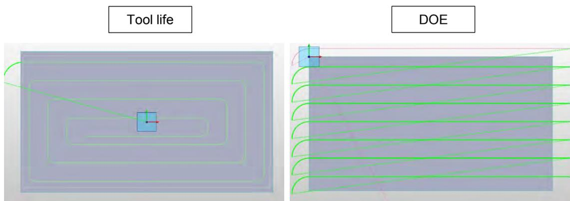
**Figure 3-4: Tool path for spiral (left) and zig-zag (right) milling (17; 18)**
