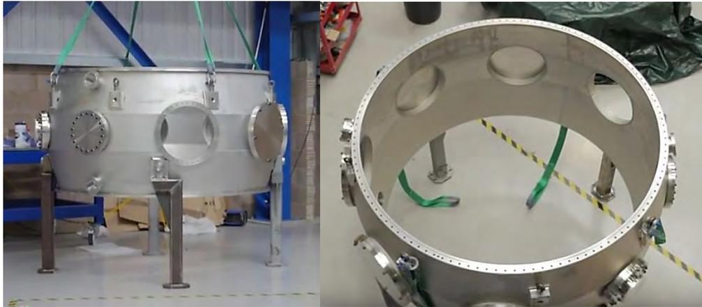
Figure 16: The core shell of the ST40 spherical tokamak's vacuum vessel [18]
