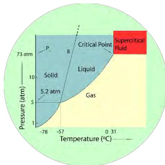
**Figure 3-2: High-pressure scCO<sub>2</sub> system with MQL (left) and temperature-pressure diagram for CO<sub>2</sub> (right) (14)**
