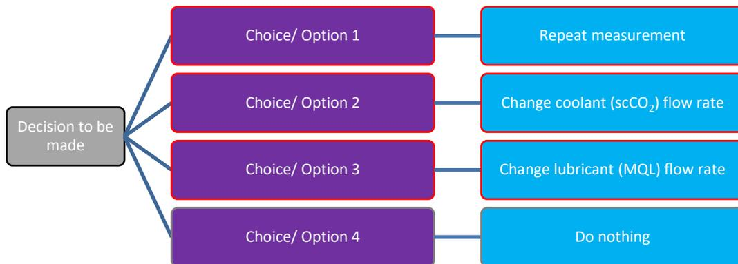
**Figure 3-8: Decision tree in optimisation of cutting conditions after reviewing the results of tool life trials**
