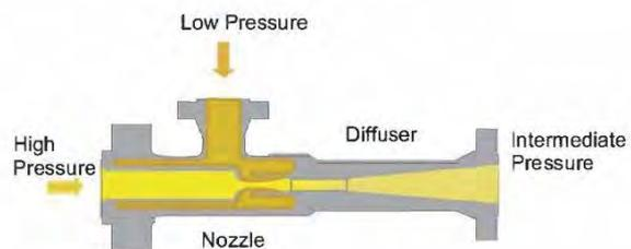
Figure 27: A typical steam jet injector
