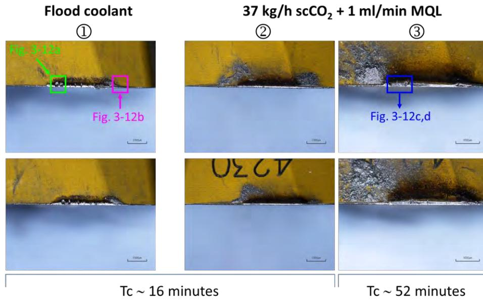
**Figure 3-11: Tool wear on the flank face of the cutting tool in due cutting time (after 16 minutes and 52 minutes)**
