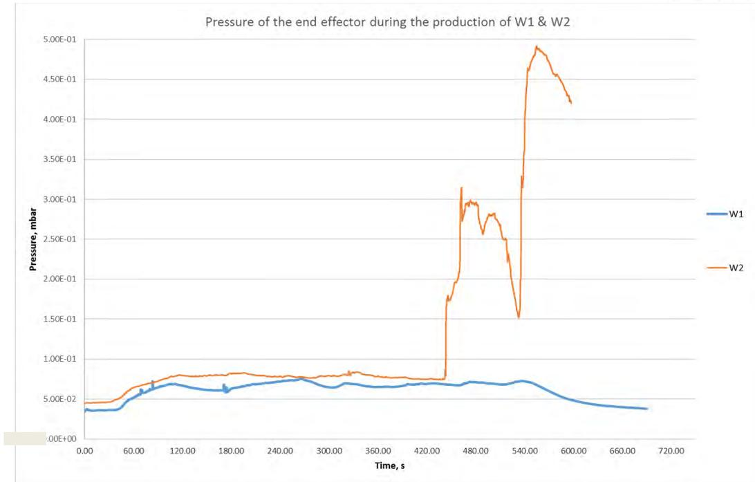
**Figure 13 Pressure in the end effector/mock vessel during the production of W1 and W2.**
