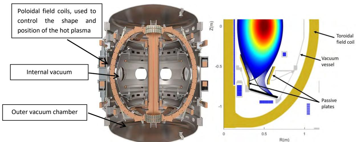
Figure 9: The ST40 spherical tokamak [10]
