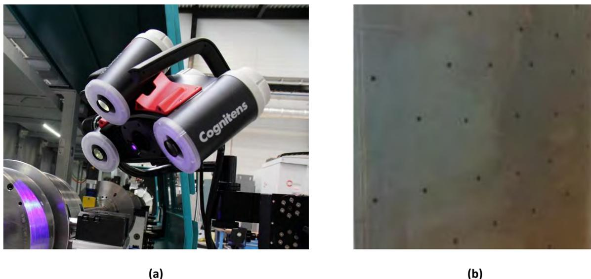
**Figure 2-12 – Photogrammetry technology: (a) Cognitens WLS400M; (b) Photogrammetry targets applied to a body panel in preparation for scanning.**
