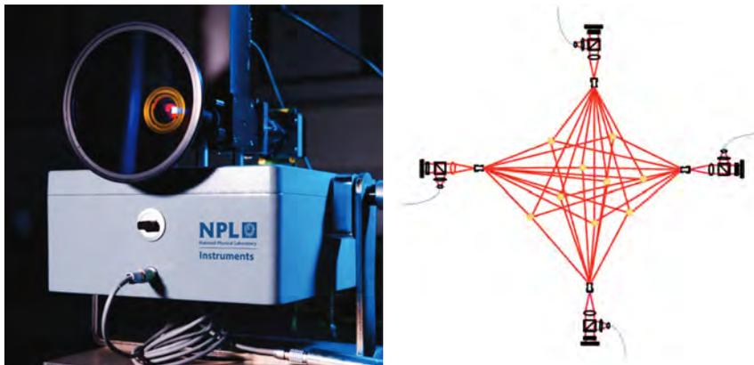
**Figure 3-3: (left) NPL FSI; (right) Developments in multi-target, wide angle, frequency scanning interferometry for coordinate measurements by multilateration<sup>20</sup>**
