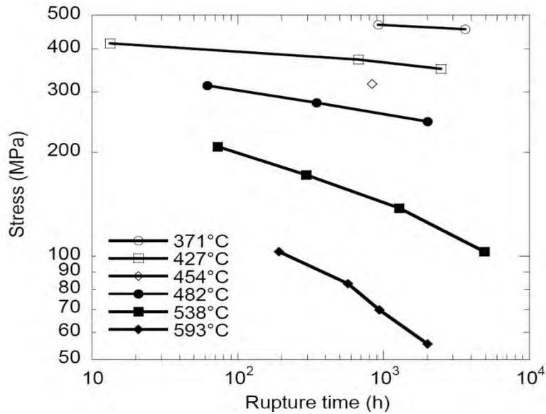
Figure 38: Creep response of SA-508 in the range 371-593°C [66]
