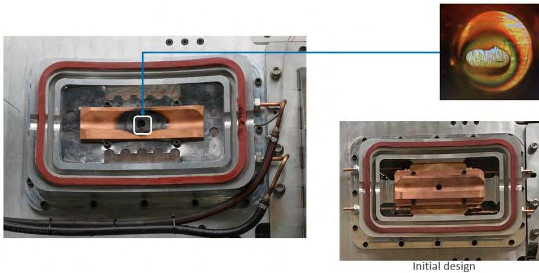
**Figure 14 Welding station with improved spatter guard and plumbing arrangement.**
