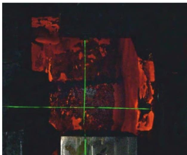
Figure 57: Projection of green laser on a hot forging
