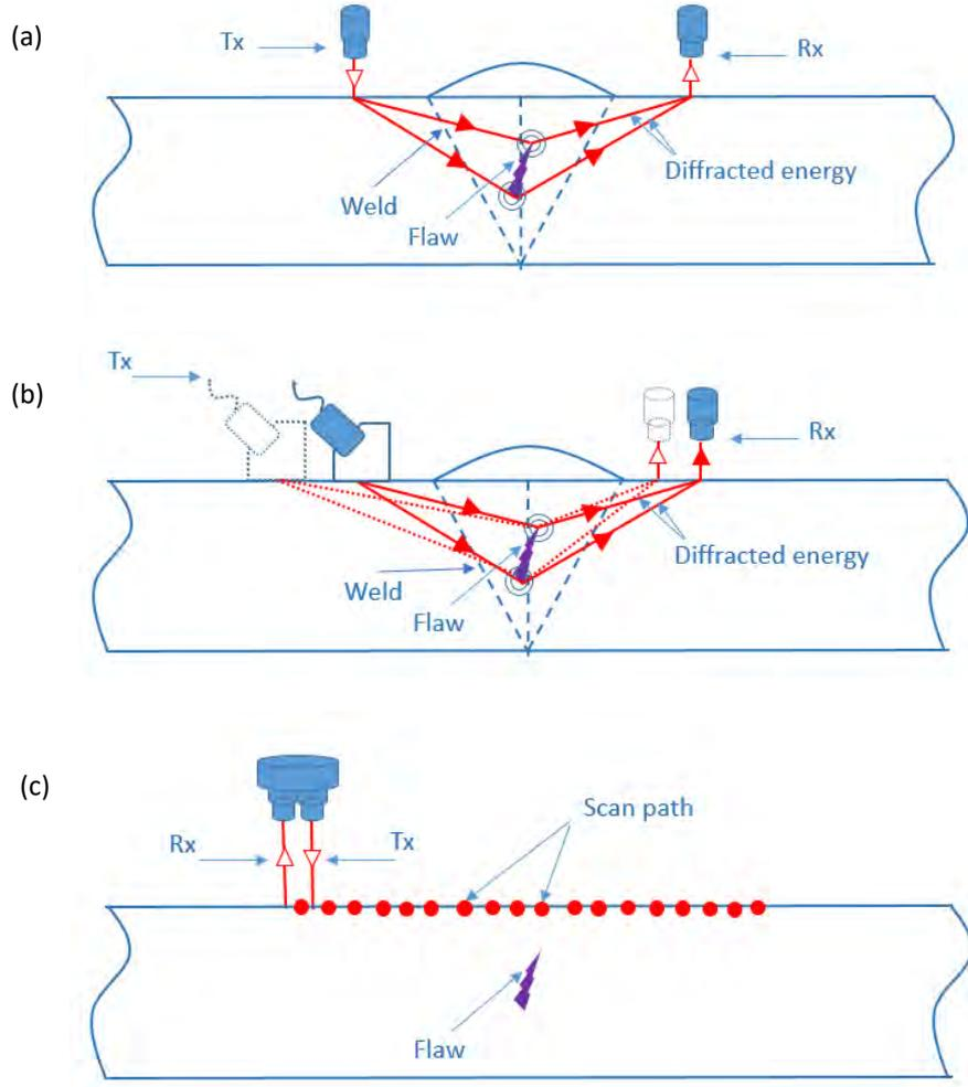
**Figure 7-2: Potential NDE development and automation during Phase II (a) TOFD using laser ultrasound (b) Hybrid Piezo-laser ultrasound (c) Dual laser ultrasound thickness measurements**
