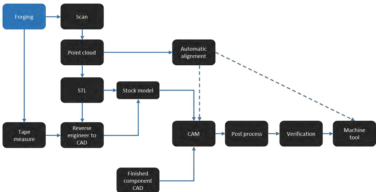
**Figure 3-7: Generic machining workflows**
