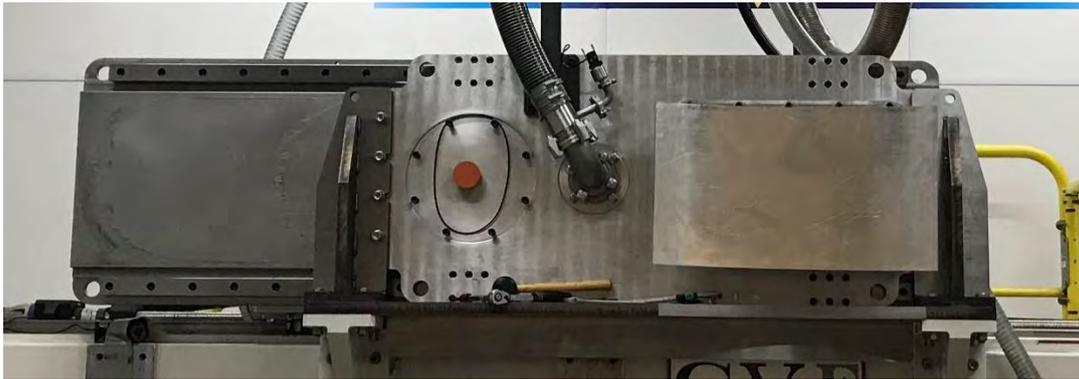
**Figure 4 Set up of static vacuum test, showing how a plate and a rubber stopper were used to blank off the welding station and the QA station.**
