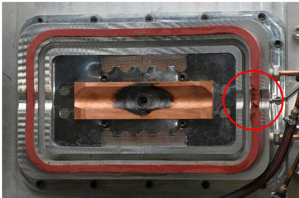
**Figure 16 Condition of the seal immediately after W2, showing significant damage on the trailing side**
