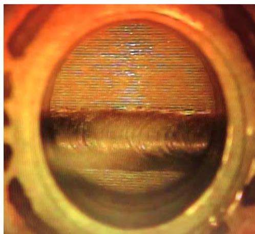
**Figure 7 Operator's view through the beam impingement camera, mounted on the column of the EB gun.**
