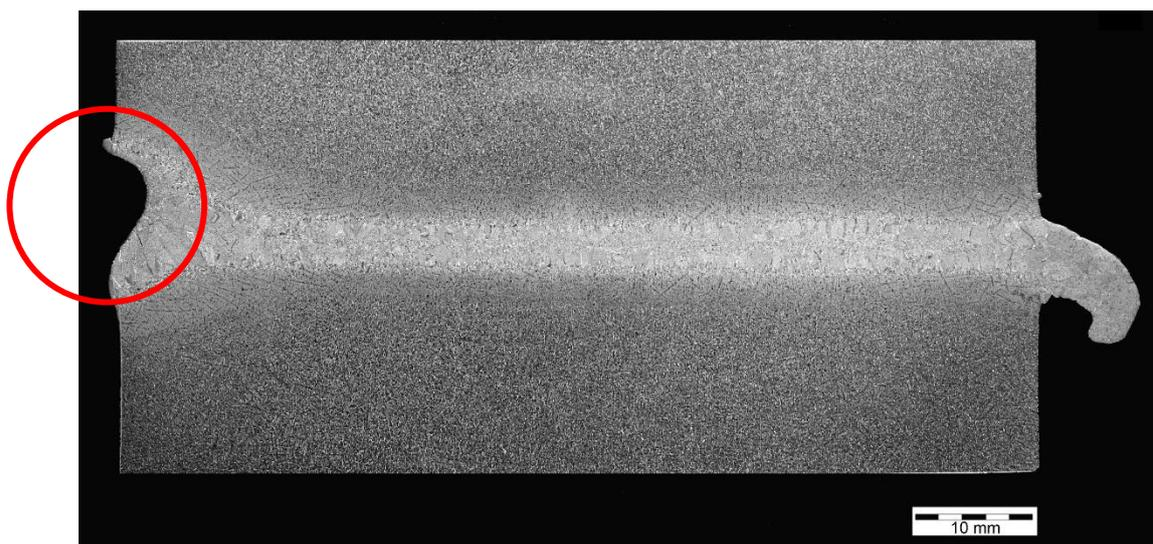
Figure 12 Macro photograph of section taken from the slope-out area of W2, with significant under-fill at the cap of the bead highlighted in red.
