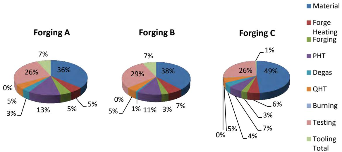
Figure 67: Percentage of cost of each manufacturing process for different forgings in Sheffield Forgemasters
