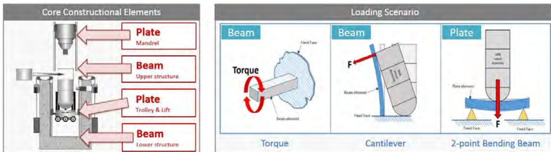
Figure 4 – Core Elements and Loading Scenarios for the Proposed InFORM Fixture
