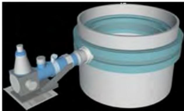
**Figure 4 Local vacuum vessel with static seals mating with pressure vessel and engineered sliding seals. Internal box seal containing beam stopper. Shown here welding in the 2G orientation, with the gun static and the vessel rotating.**
