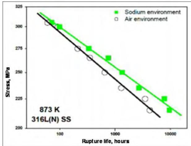
Figure 35: Enhanced creep rupture of 316L(N) SS in sodium environment [51]
