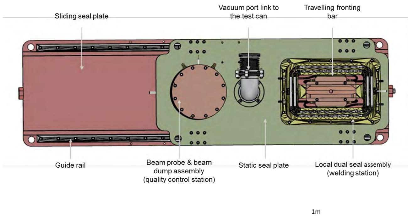
**Figure 1** *The final design of the end effector unit with description of the primary elements.*
