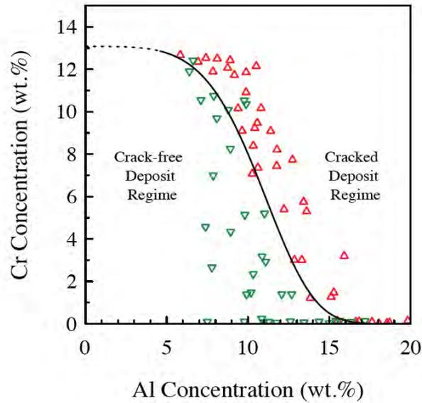
Figure 29: Cracking susceptibility map for weld overlays in FeCrAl alloys. Reproduced from [41]
