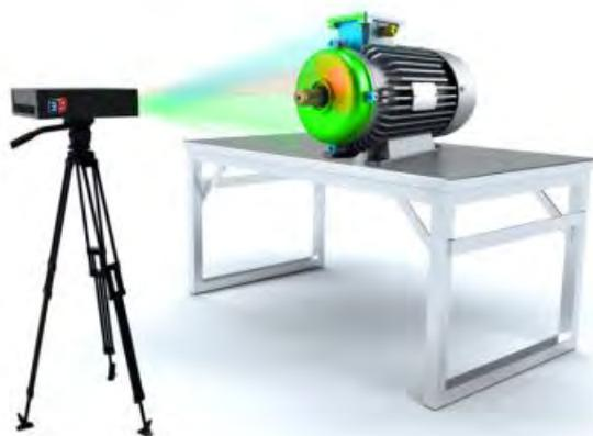
**Figure 2-14:** Illustration of how colour map data is displayed on a part by projection.
