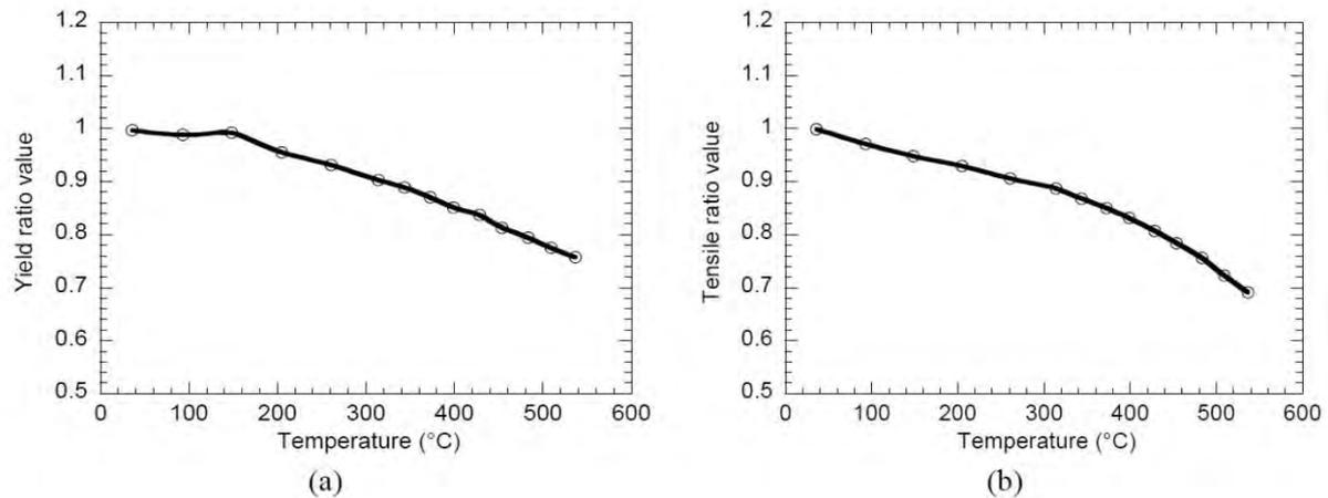
Figure 39: Ratio trend curves of YS and UTS ratio as a function of temperature (a) YS and (b) UTS
