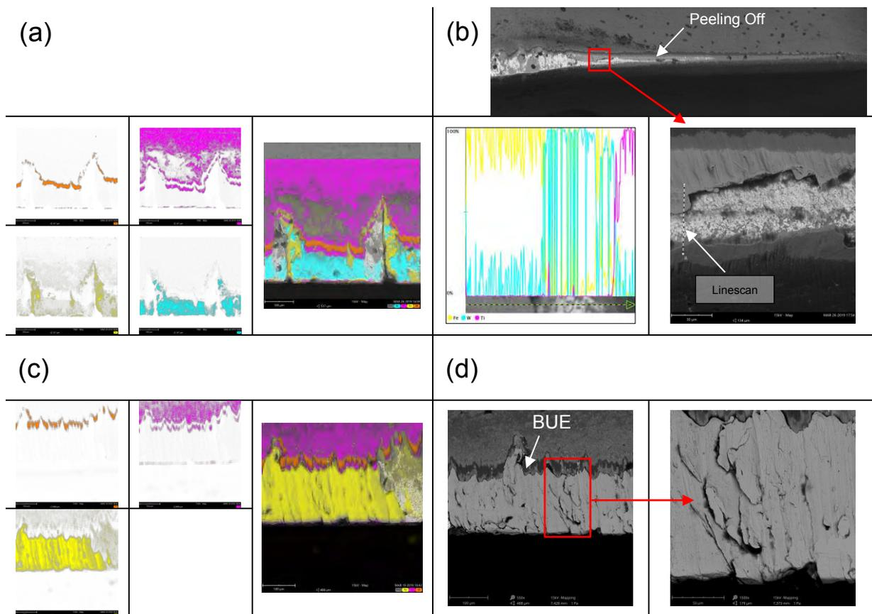
**Figure 3-12: SEM/EDS elemental mapping (a, c) and line concentration profile (b) on the tool flank face after milling with flood coolant (a, b) and sCCO<sub>2</sub>+MQL (c, d)**
