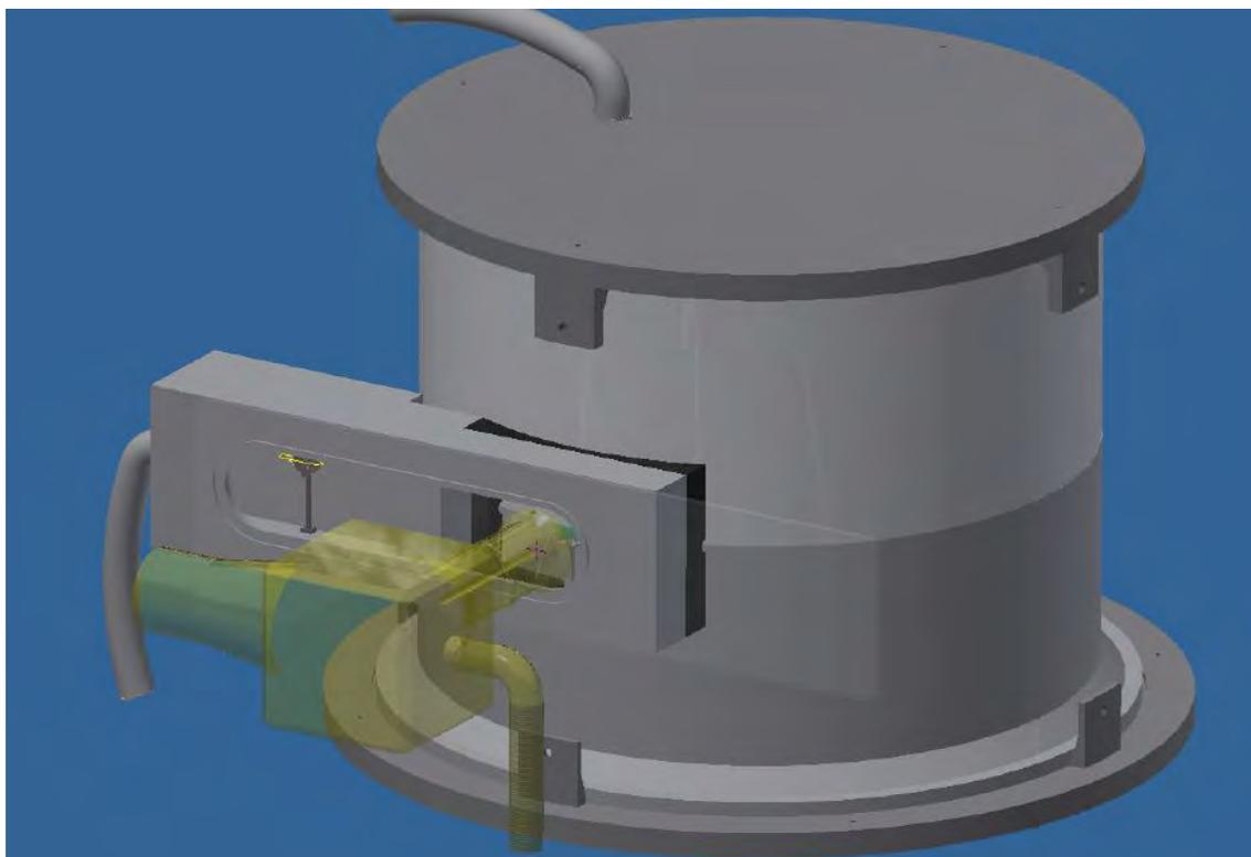
**Figure 2 Alternative view of assembly with gun positioned for welding.**
