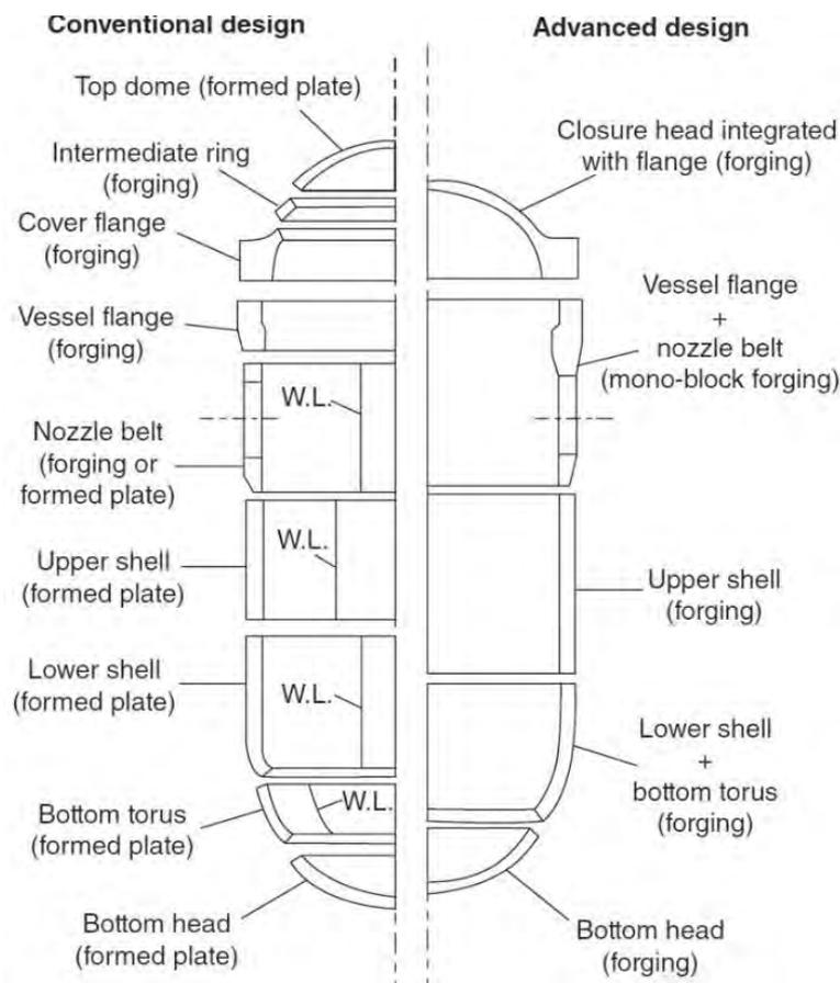
Figure 46: Layout of conventional and advanced type reactor pressure vessel [15]
