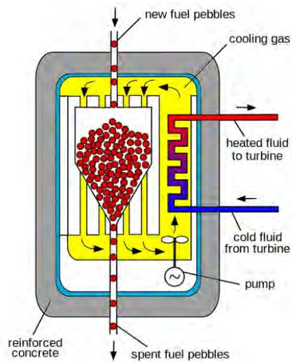
Figure 7: Pebble Bed Reactor scheme [8]
