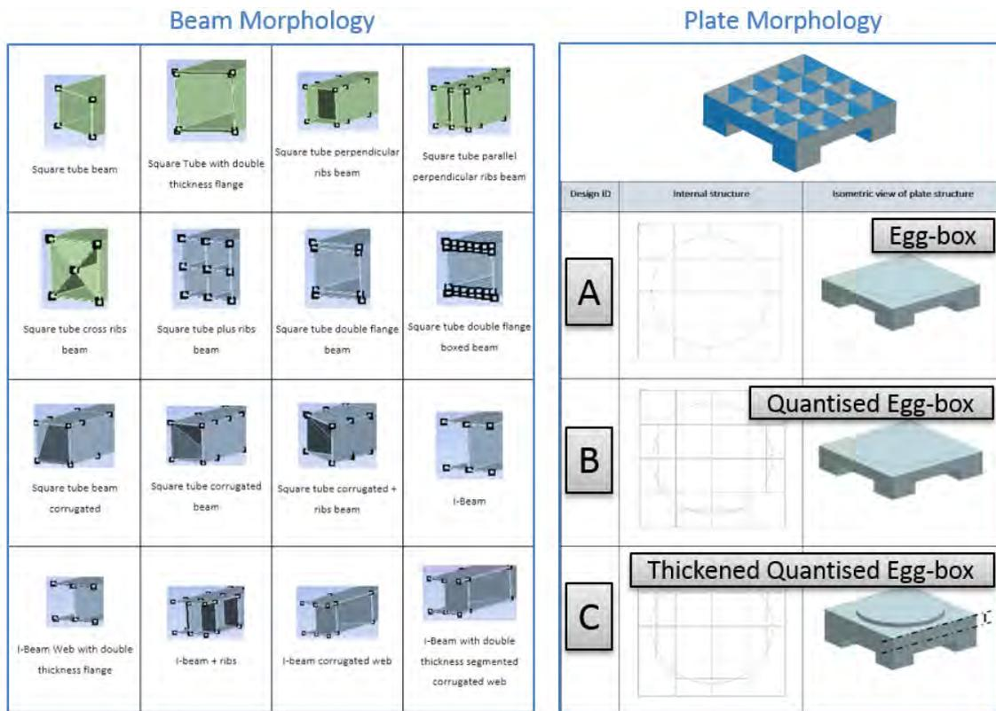
Figure 5 – Proposed Beam and Plate Structural Morphologies
