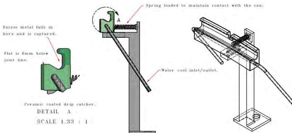
**Figure 6 Travelling fronting bar concept.**
