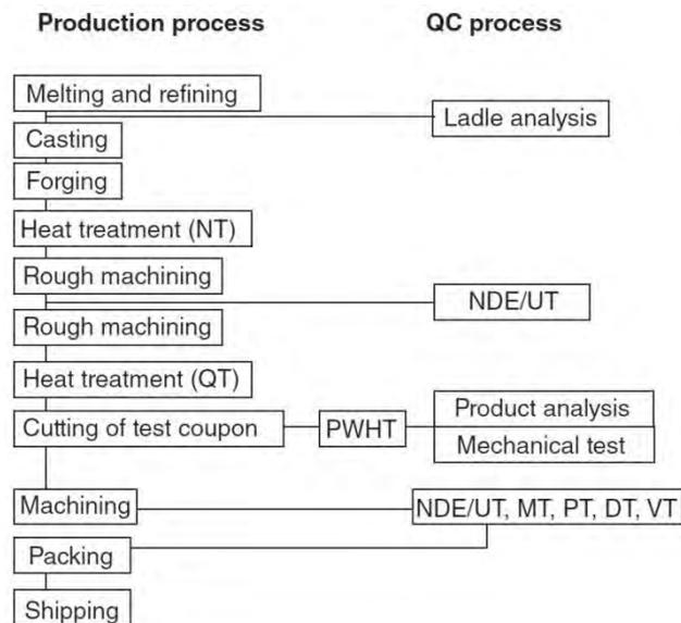
Figure 45: Typical manufacturing sequence of an RPV component (shell). UT, ultrasonic test; DT, dimensional test; MT, magnetic particle test; VT, visual test; PT, liquid penetration test; NDE, non-destructive examination; PWHT, post-weld heat treatment [15]
