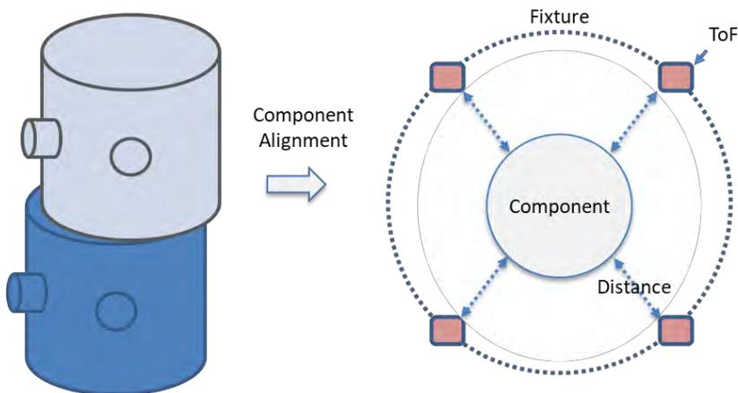
Figure 2: InFORM component alignment concept
