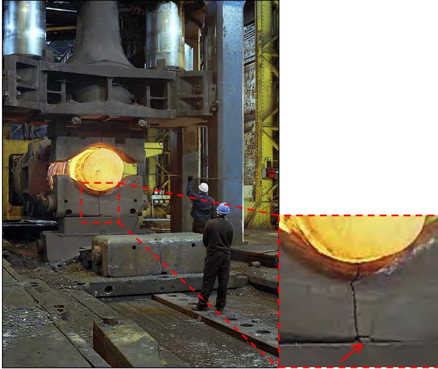
Figure 63: Damage on forging tools due to heavy loading and the existence of stress concentrations which promote the initiation and propagation of cracks
