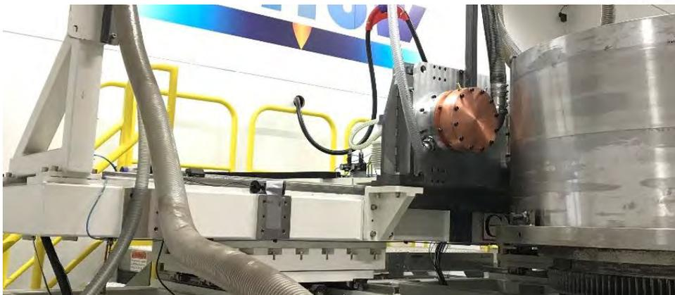
**Figure 5 End effector operating in welding position during dynamic vacuum tests.**
