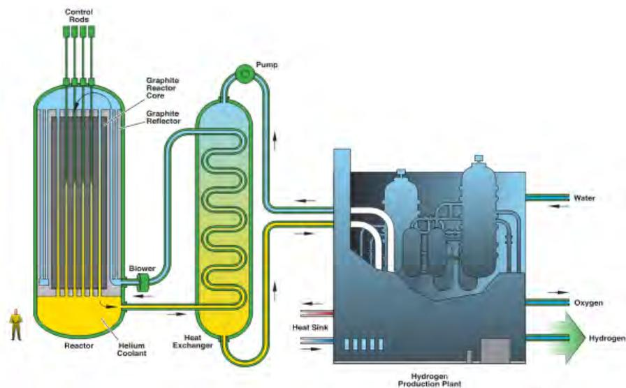
Figure 6: The Very High Temperature Reactor (VHTR) [7]
