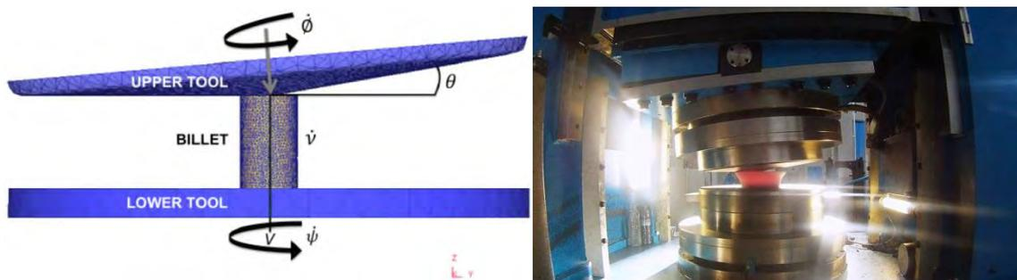
Figure 66: The rotary forging process
