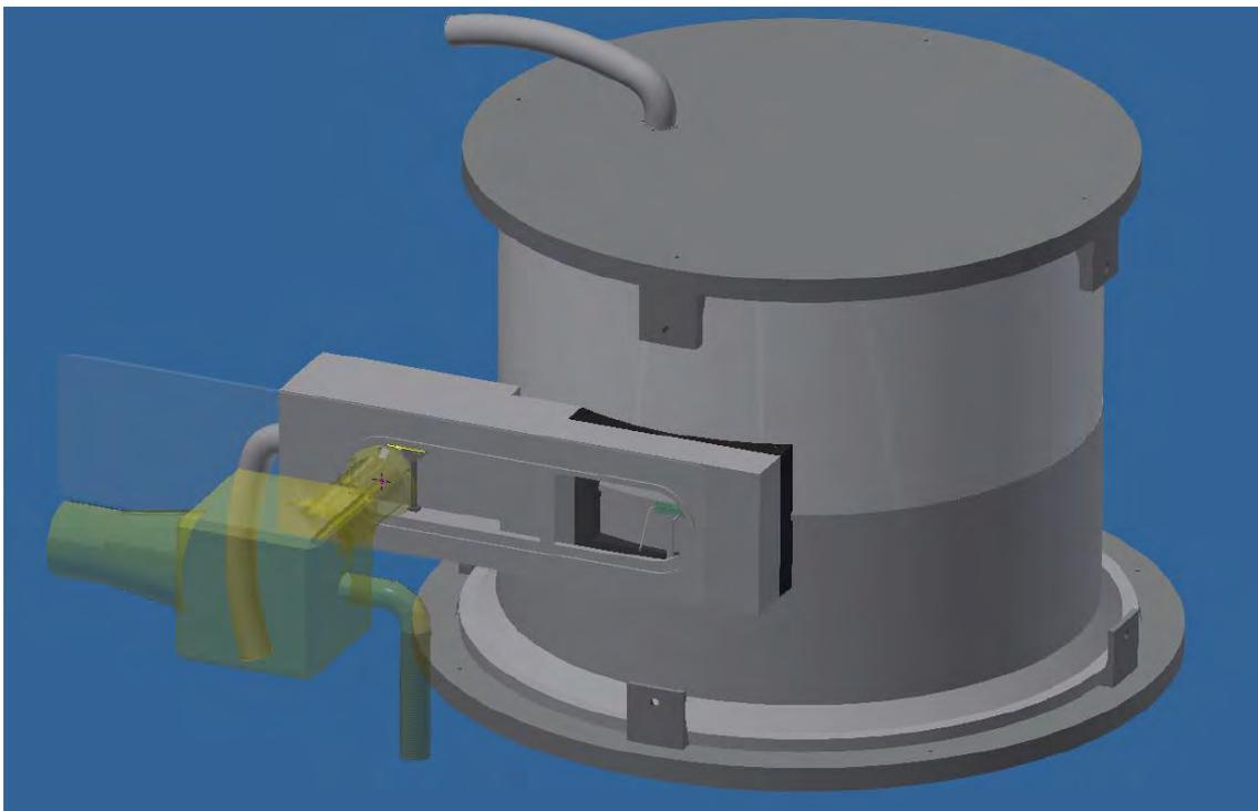
**Figure 1 Overview of concept assembly with gun positioned for pre-weld conditioning.**
