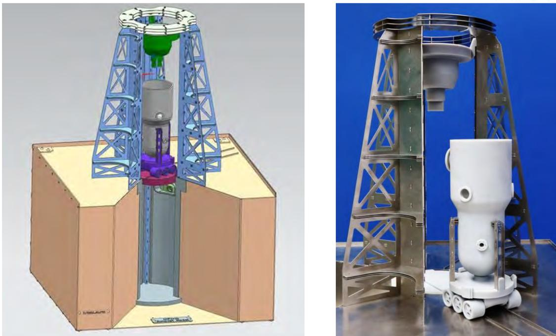
**Figure 4-3: MetLase fixture concept: Left, CAD model; Right, physical model (displayed at Nuclear AMRC)**
