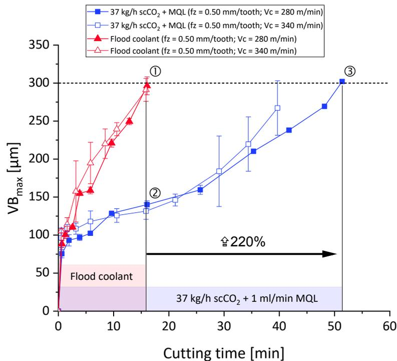
Figure 3-10: Tool life in the milling of SA508 steel (Grade 3 Class 2)
