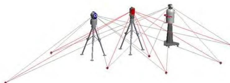
**Figure 5-1: Unified Spatial Metrology Network (USMN), a function within Spatial Analyser, accurately determines the position of common points relative to each other using measurements of those common points from different instrument stations**
