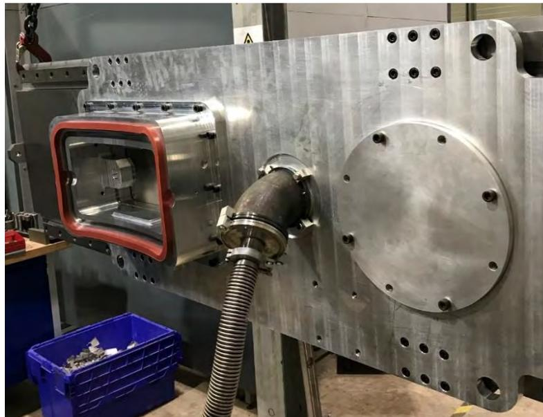
**Figure 5 Static seal plate with the local dual seal unit, without the travelling fronting bar or beam dump in place, and showing temporary pumping pipe.**
