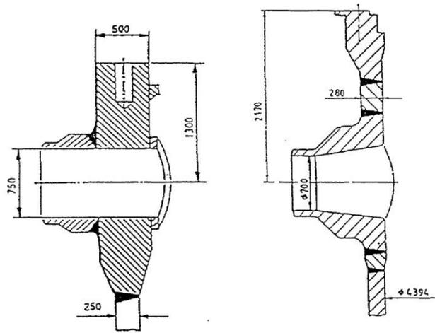
Figure 12: Sketches of typical set-on and set-in nozzles used in reactor pressure vessel [11]
