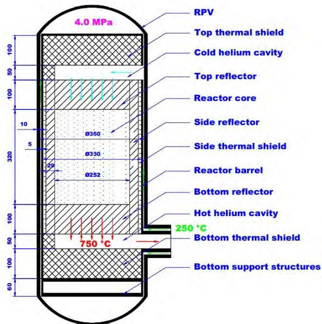
Figure 15: Reactor Pressure Vessel and Core Internals of a VHTR [17]
