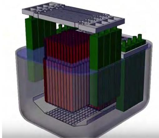
Figure 4: The stable salt reactor core, with support structures in grey
