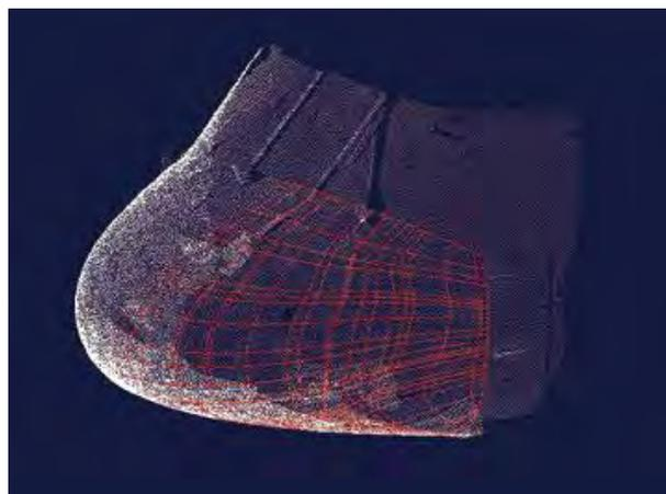
**Figure 1-2: Nose – ATOS scan data (optical white light scanner data) (5)**
