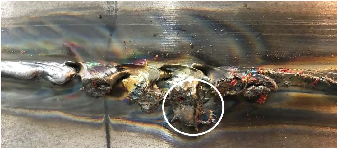
**Figure 17** *Bead cap of W3, showing the drip catcher had caught, formed and solidified the molten drips, preventing their progression.*
