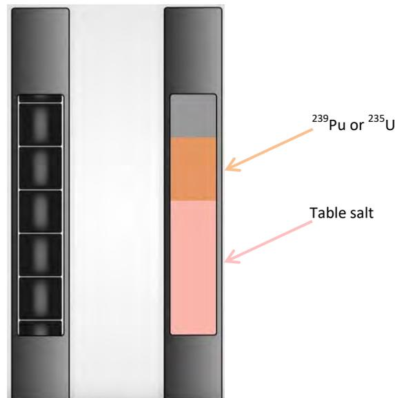
Figure 5: Replacement of pellets (left) with liquid molten salt which contains the nuclear fuel (right) [6]
