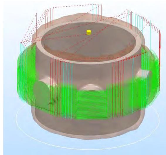
**Figure 3-14: Toolpath simulations in Vendor A**
