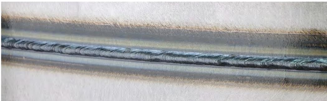
**Figure 8 Appearance of the cap bead of W1.**
