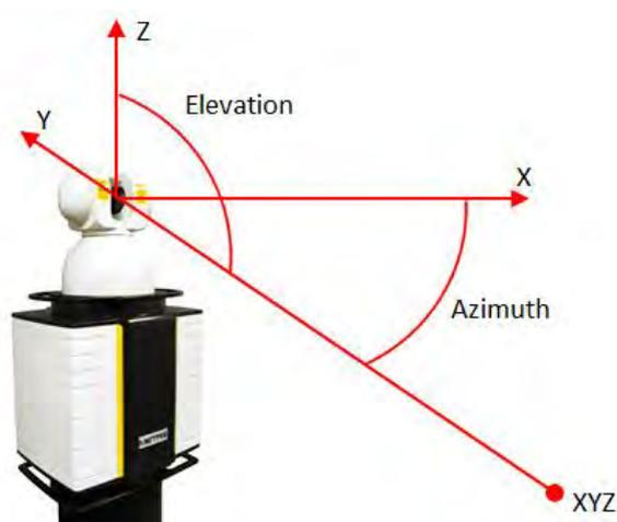
Figure 2-2 - Nikon Laser Radar, coordinate system
