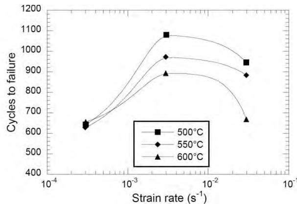
Figure 43: Effect of strain rate on the low cycle fatigue behaviour of modified 9Cr-1Mo steel in air [72]
