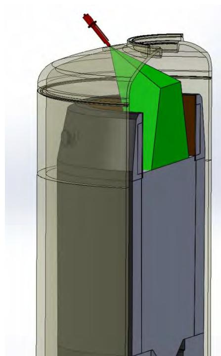
Figure 23: CAD model of a possible field of view (green volume) using an IR camera during VSD
