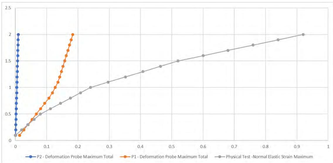
Figure 11 – FEA Tensile Comparison Study for ML Fastener – Grey: Physical Test,
