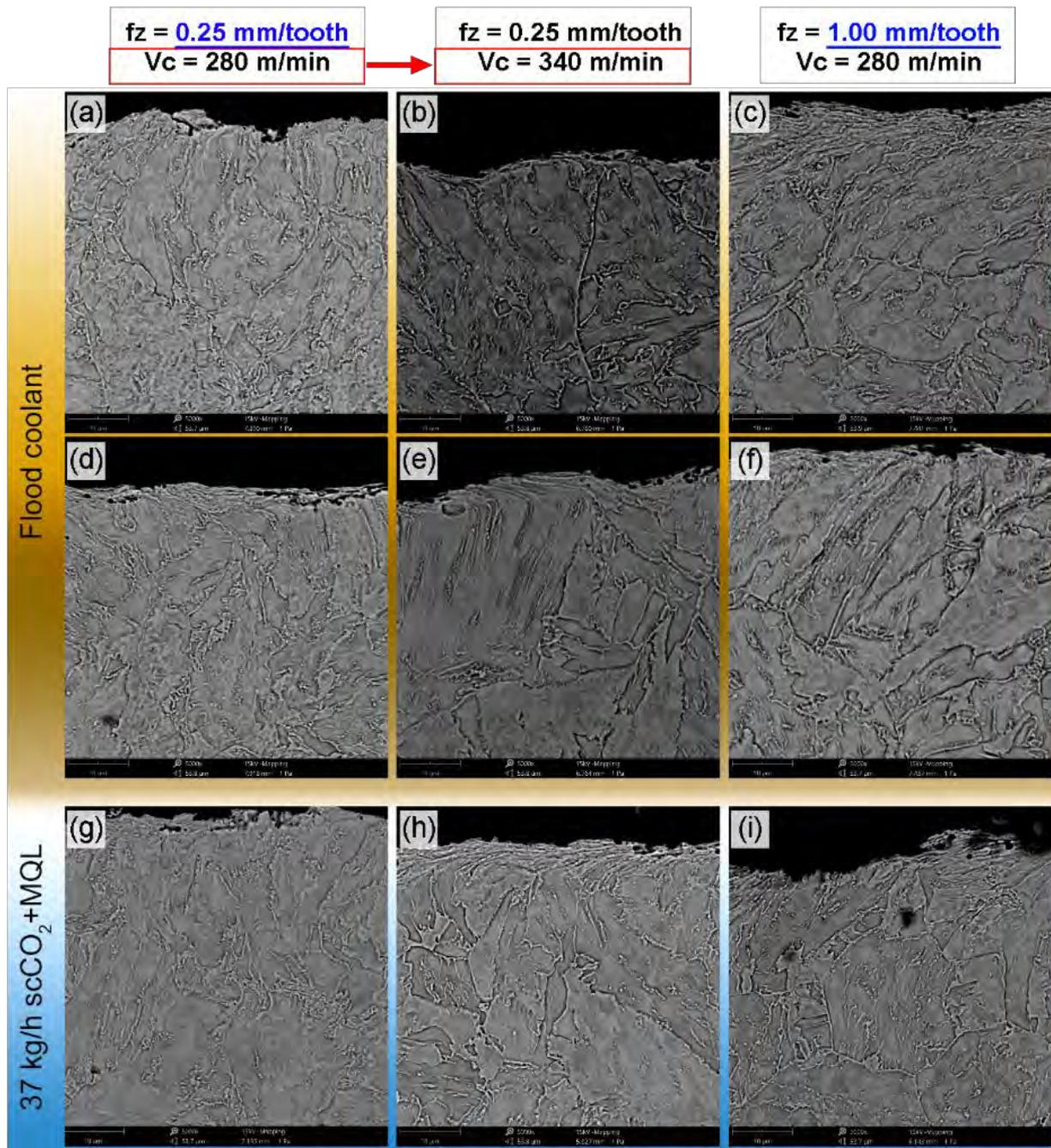
Figure 3-21: SEM micrographs (x5000) of the microstructures in the transverse direction
