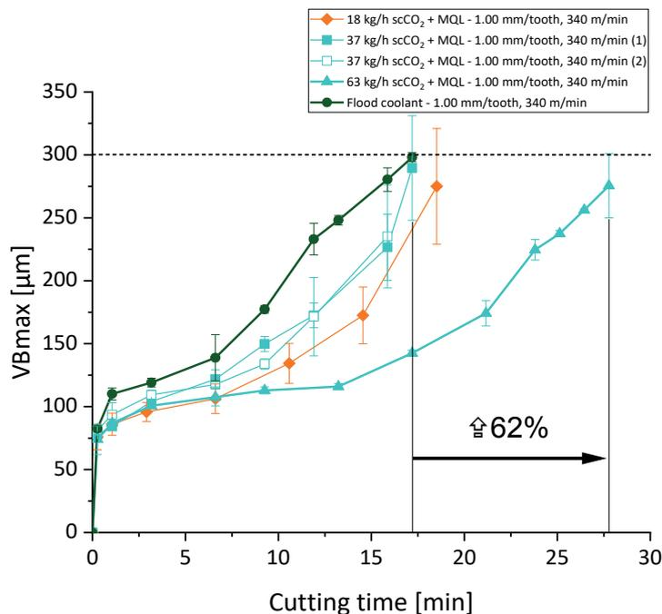
**Figure 3-9: The influence of scCO<sub>2</sub>+MQL flow rate on tool wear at the highest levels of cutting conditions**
