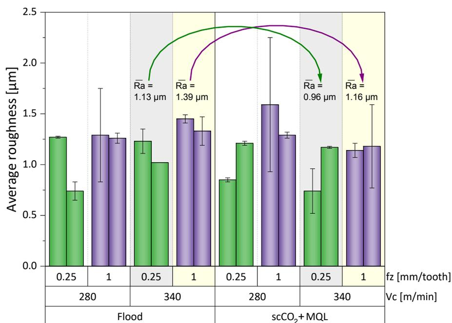
Figure 3-13: Surface roughness (Ra values) for SA508 steel after milling with flood coolant and  $scCO_2+MQL$
