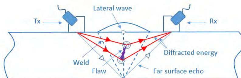
**Figure 7-1: Schematics of conventional TOFD technique**
