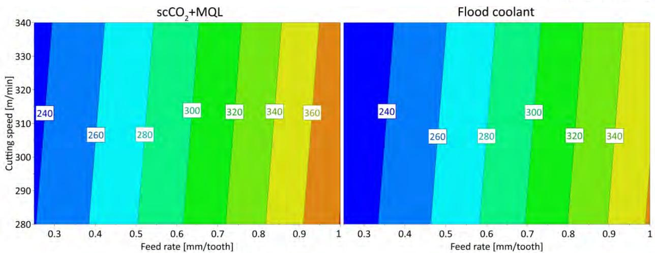
**Figure 3-15: Response contour plot of feed force in milling SA508 steel with scCO<sub>2</sub>+MQL (left) and flood coolant (right)**
