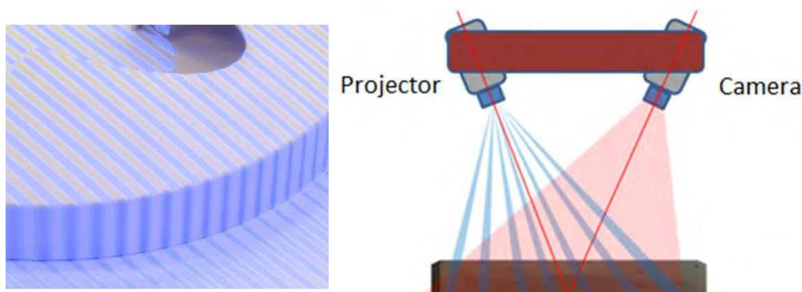
**Figure 2-5 - The relationship of fringe pattern projection and camera image capture**
