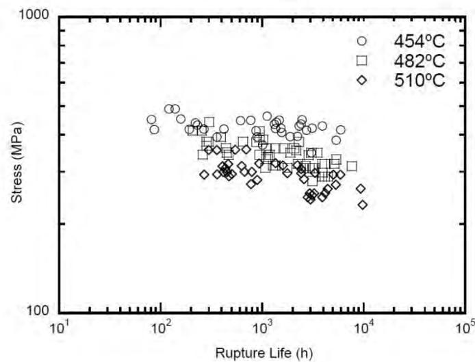
Figure 40: Creep rupture behaviour of 2.25Cr-1Mo-0.25V steel at different temperatures [68]
