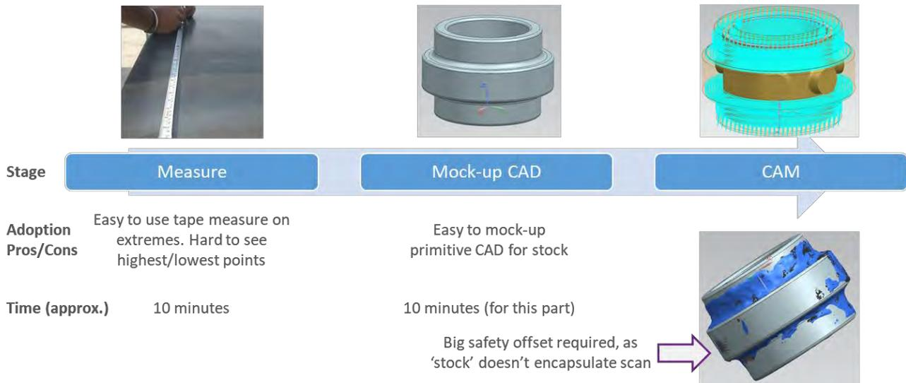
**Figure 3-8: Typical procedure for traditional (simple) reverse engineering**
