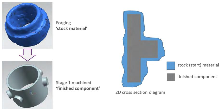
**Figure 3-2: Forging test model**
