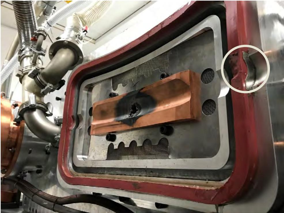
**Figure 15** *Condition of the seal immediately after W1, showing no visual damage, with the lead in and the shim highlighted in white.*
