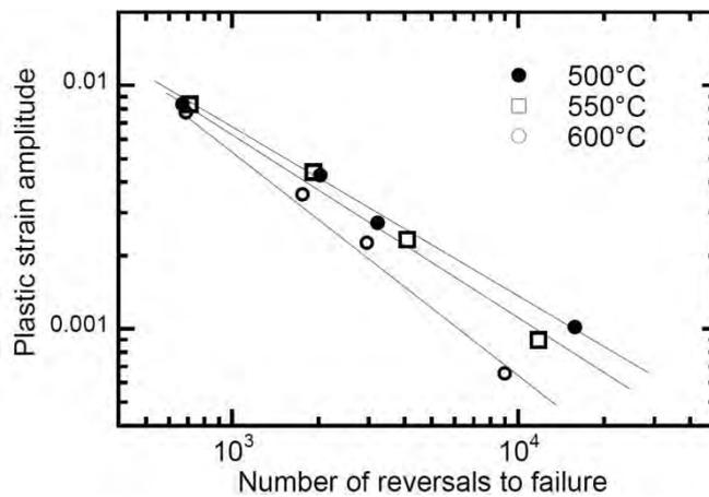
Figure 42: Low cycle fatigue life of modified 9Cr-1Mo steel in air at various test temperatures [72]
