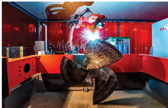
**Figure 1-3: Wire Arc Additive Manufacture (WAAM) of a ship propeller blades (7)**
