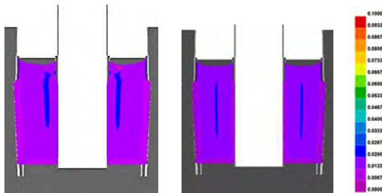
Figure 51: Predicted porosity pattern of the 1950's hollow ingot method (left) and today's method (right)
