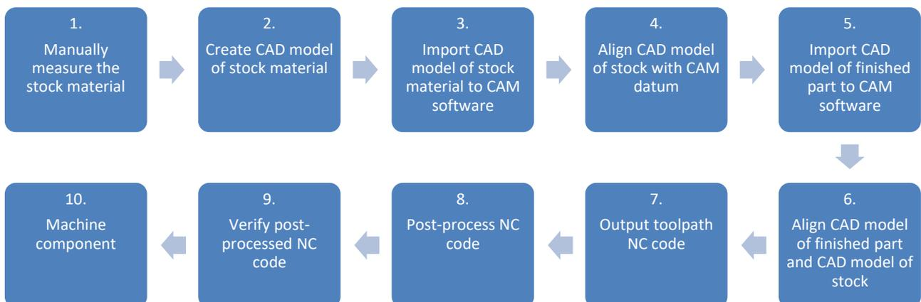
**Figure 3-9: Traditional (simple) reverse engineering workflow stages**
