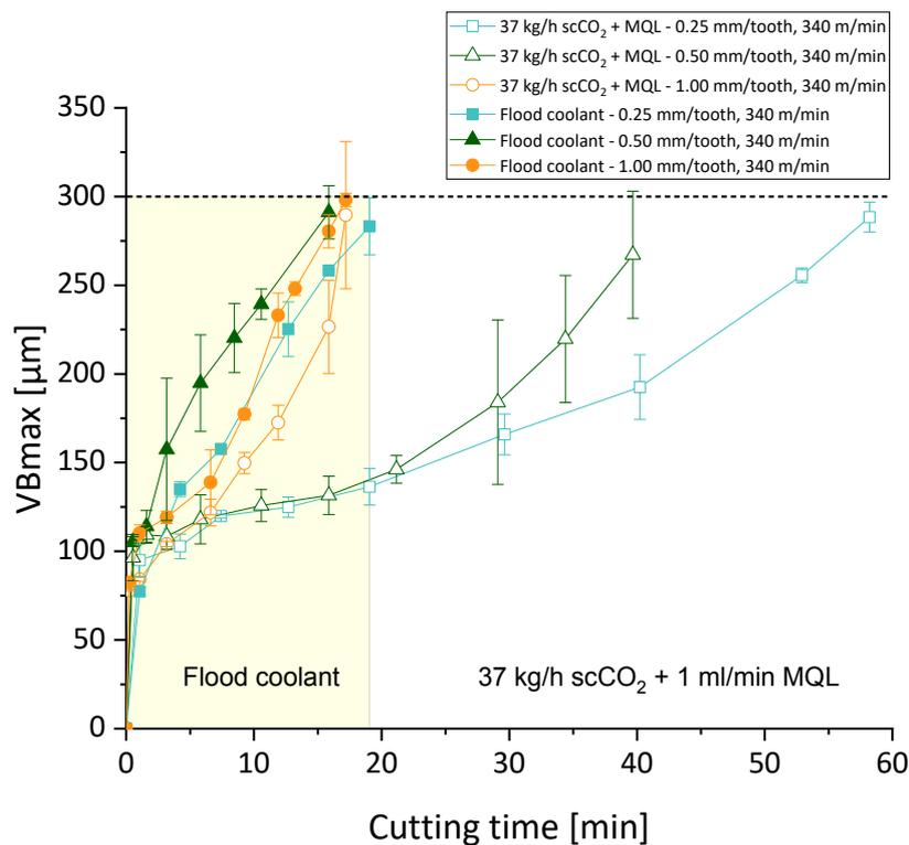
**Figure 3-7: Maximum flank wear ( $VB_{max}$ ) as a function of cutting time at various feeds and cutting speed of 340 m/min**
