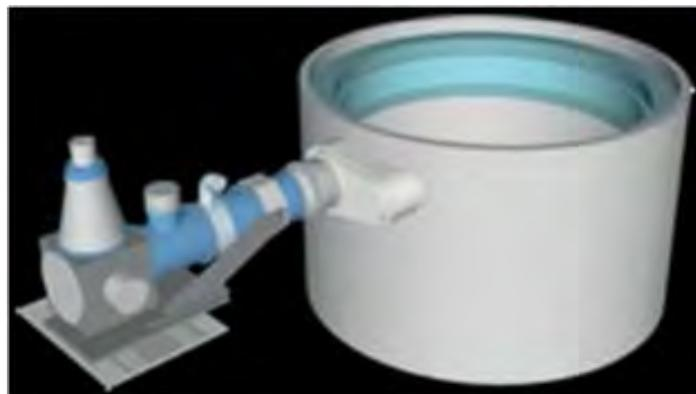
**Figure 2** Local vacuum sliding head mounted on gun column and internal box seal containing beam stopper. Shown here welding in the 2G orientation, with the gun static and the vessel rotating.
