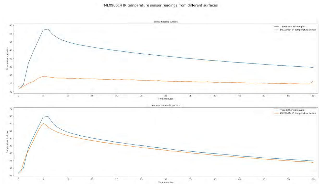
Figure 19 : IR Temperature measurement variation by target surface
