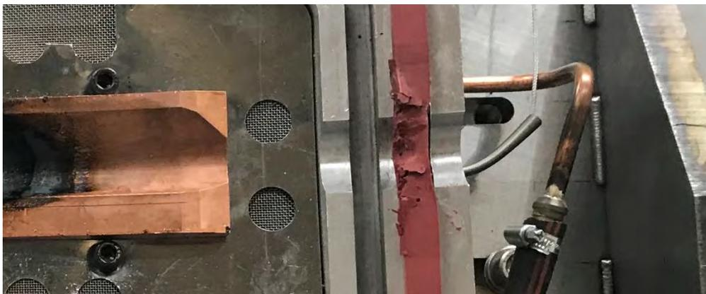
**Figure 19** *Condition of the seal immediately after W3, showing extensive damage caused by the ragged bead.*
