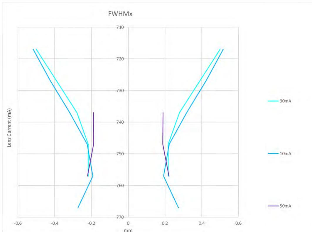
**Figure 20 Lens current vs FWHM X.**
