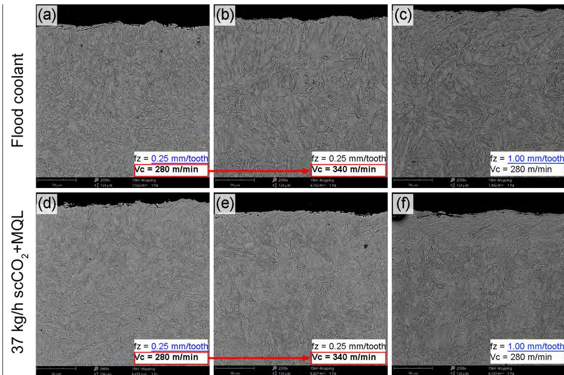
Figure 3-20: SEM micrographs (x2000) of the microstructures in the transverse direction
