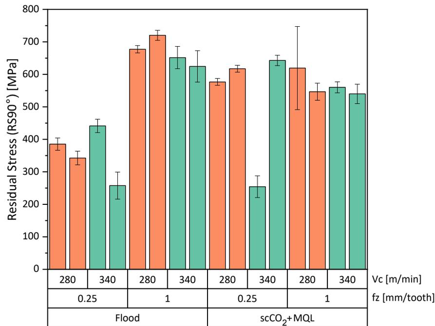
**Figure 3-17: Residual stress in the transverse (top) and longitudinal (bottom) directions after milling of SA508 steel**
