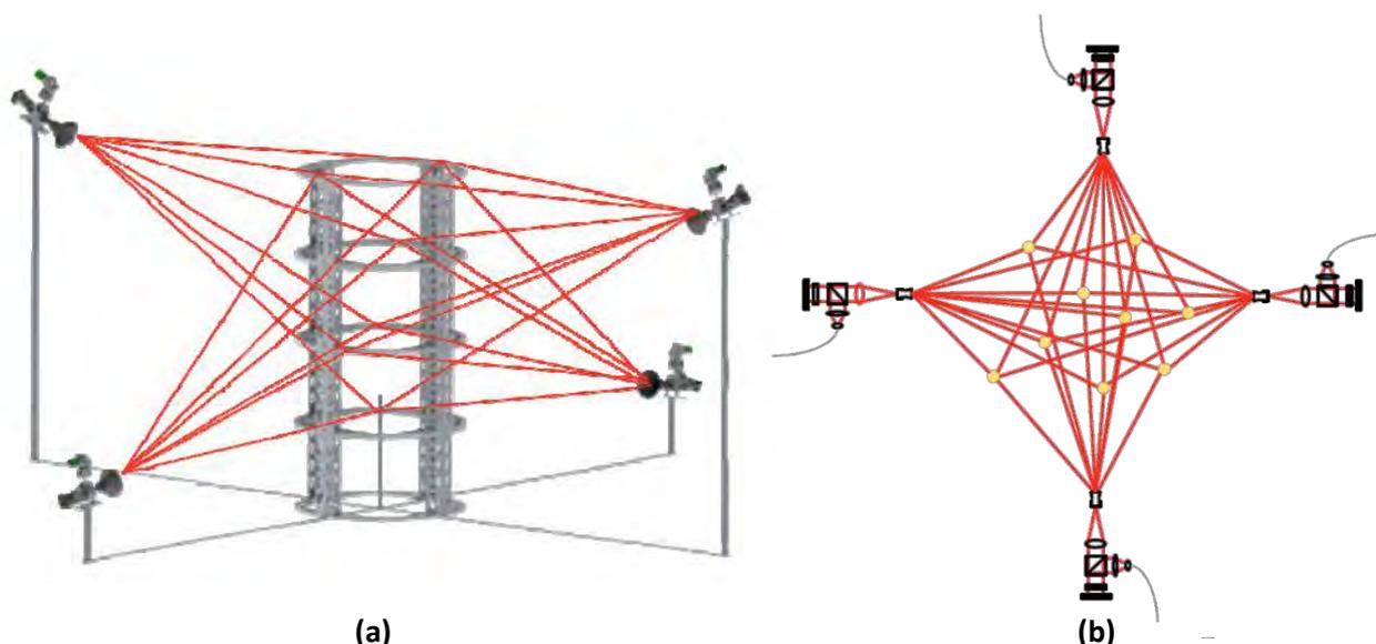
Figure 2-13: A multilateration system composed of 4 sensors in (a) 3D and (b) aerial views.
