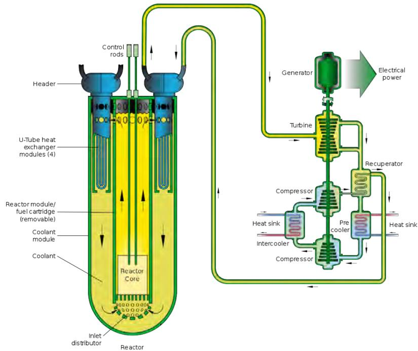
Figure 1: Schematic of the lead-cooled fast reactor [4]
