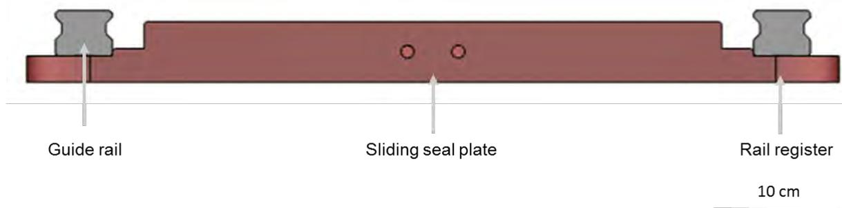
Figure 7 End view of the sliding seal plate, showing the guide rails and the rail registers.
