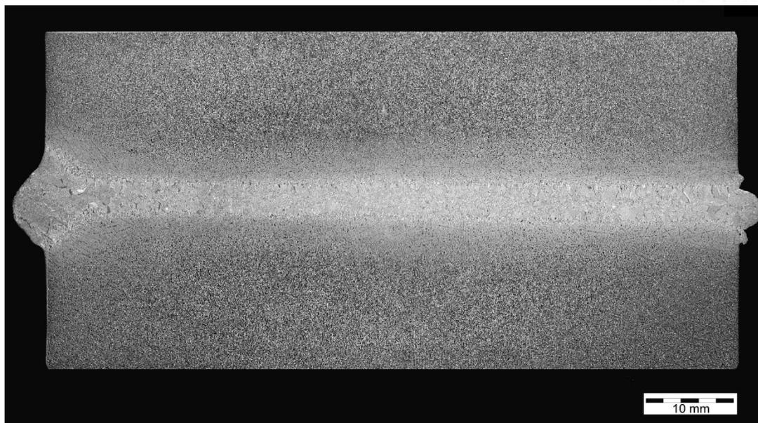
Figure 11 Macro photograph of section taken from the steady state area of W2.
