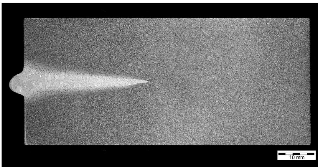
**Figure 10 Macro photograph of section taken from the slope-up area of W2.**
