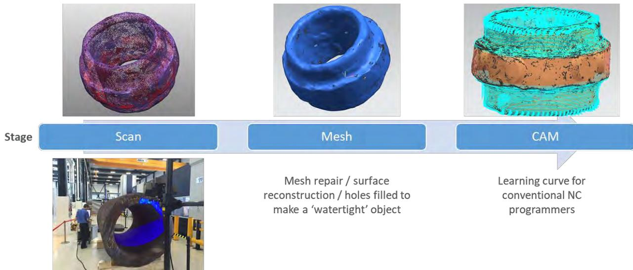
**Figure 3-12: Scan-to-CAM process**
