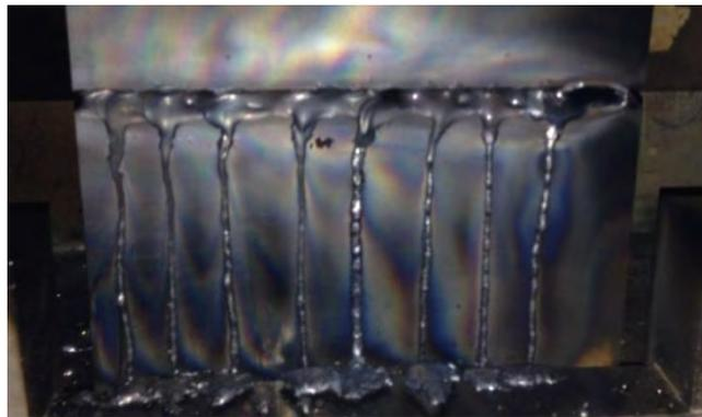
**Figure 18** *Cap of a defective weld made in 160mm thick C-Mn steel without support and with gross loss of weld metal.*
