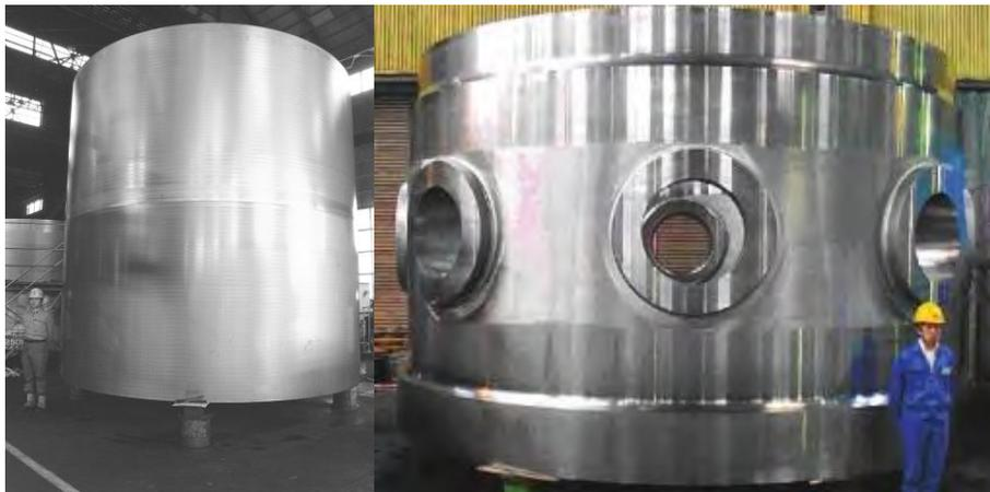
Figure 11: The core region shell (a) and the nozzle shell with integrated flange (b) of a European Pressure Reactor (EPR) [15]
