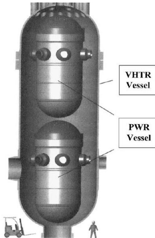
Figure 8: The pressure vessel construction envisioned for the VHTR as opposed to current typical pressurised water reactors (shown inside the VHTR vessel) [9]
