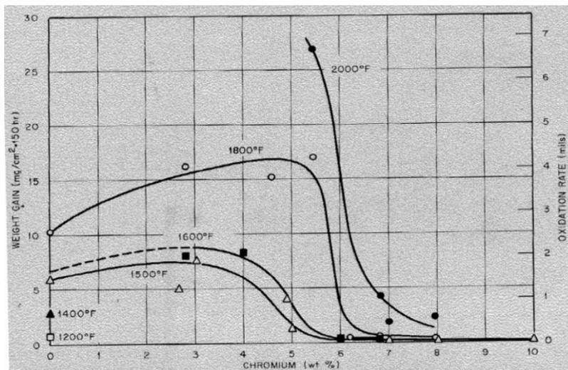
Figure 36: Oxidation rate of Ni alloys as a function of the Cr content for several temperatures [53]
