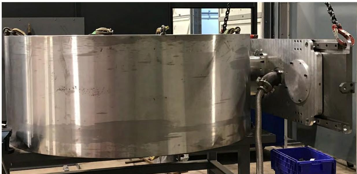
**Figure 6 Test canister (left), with the end effector (right).**
