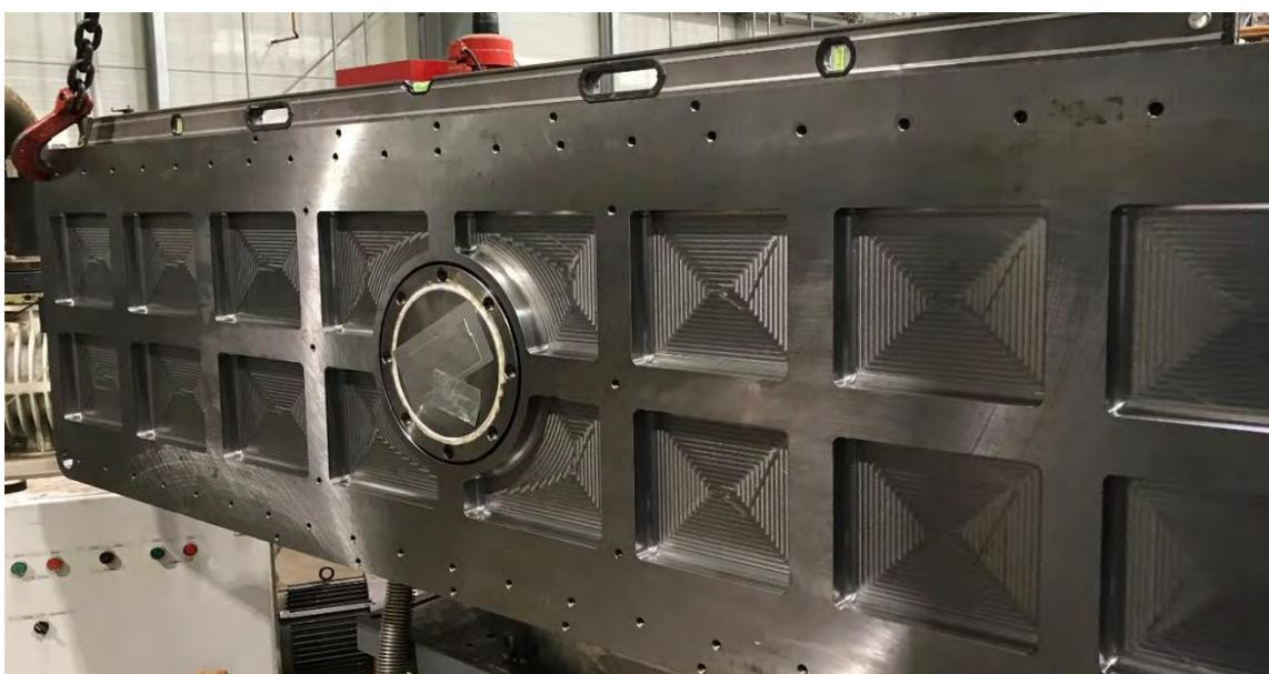
**Figure 4 Rear view of the sliding seal plate, showing gun port blanked.**
