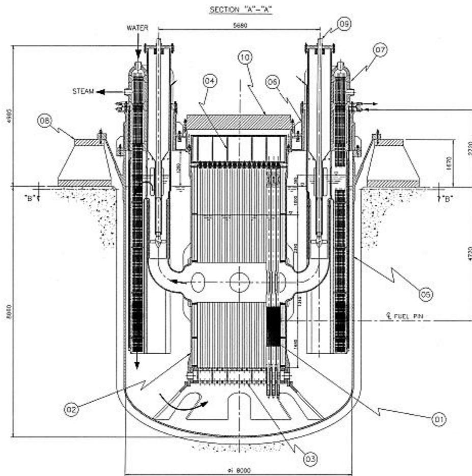
Figure 13: Advanced Lead-cooled Fast Reactor European Demonstrator (ALFRED) Reactor block vertical sections (01) Fuel assembly; 02) Inner vessel; 03) Core lower grid; 04) core upper grid; 05) Reactor vessel; 06) Reactor cover; 07) Steam Generator; 08) Vessel support; 09) Primary pump; 10) Reactor FAs cover [16]
