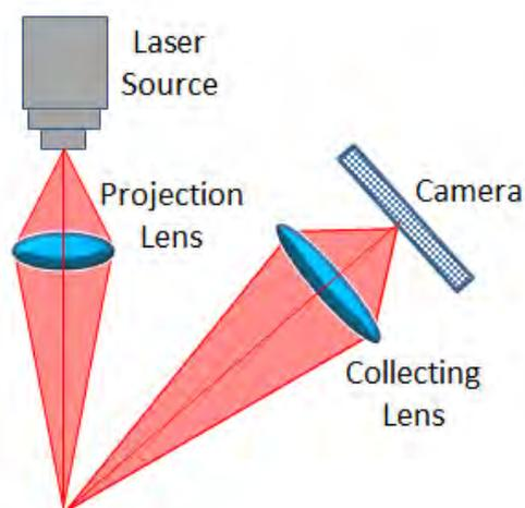
**Figure 2-7 - Laser source and receiver are mounted at a distance and angle so the path can be triangulated**
