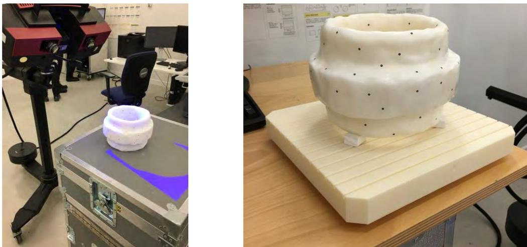
**Figure 3-15: Scanning the forging test model with GOM structured light scanner**
