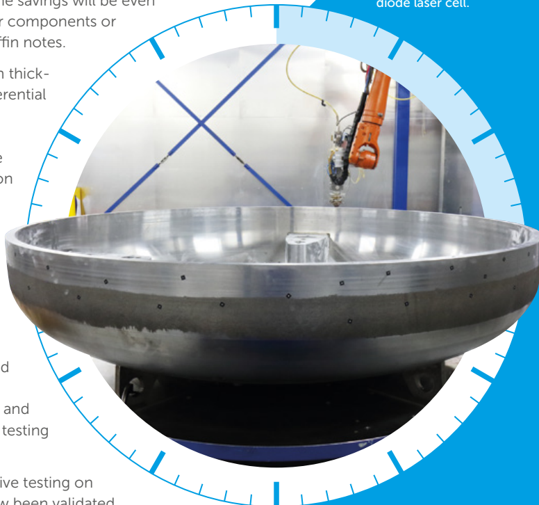
Protective cladding: a vessel dome in the diode laser cell.
