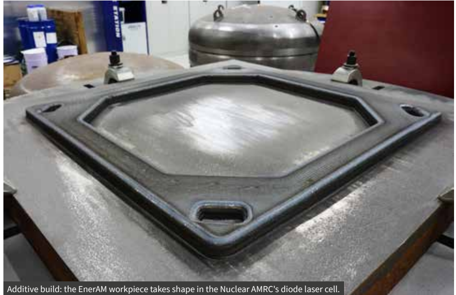
Additive build: the EnerAM workpiece takes shape in the Nuclear AMRC's diode laser cell.
