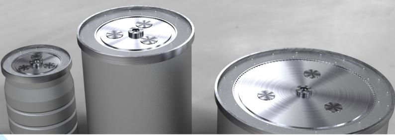
The lid uses a reverse-iris mechanism which can be operated remotely, takes less time to seal than a bolted lid, and doesn't require time-consuming inspections such as torque feedback checks to ensure the seal meets quality requirements. The design also avoids the risk of steel bolts seizing up during storage, so the lid can be easily removed if required for waste monitoring or processing.
