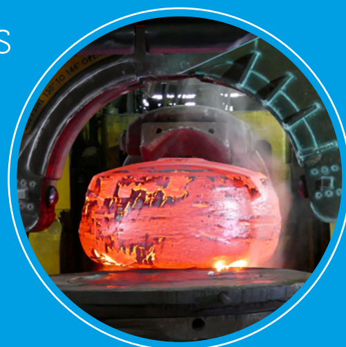
Heavy forging: demonstration pressure vessel head takes shape at Sheffield Forgemasters.
